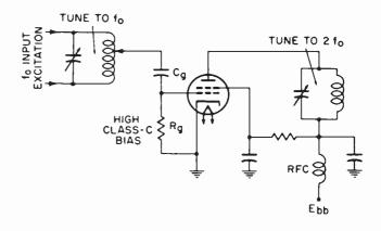
Fig. 10. Radio-frequency doubler.
