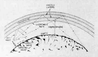
Fig. 2. Propagation of radio waves.
