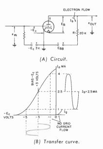
Fig. 8. Basic vacuum-tube amplifier.
