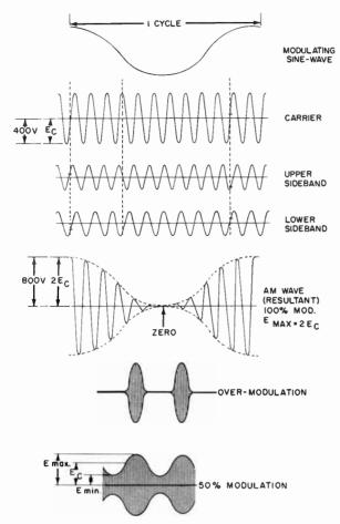
Fig. 2. Examples of AM modulation waveforms.
