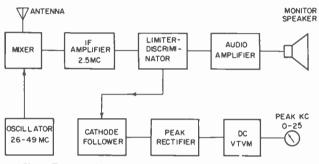
Fig. 17. Functional plan of Lampkin modulation meter.
