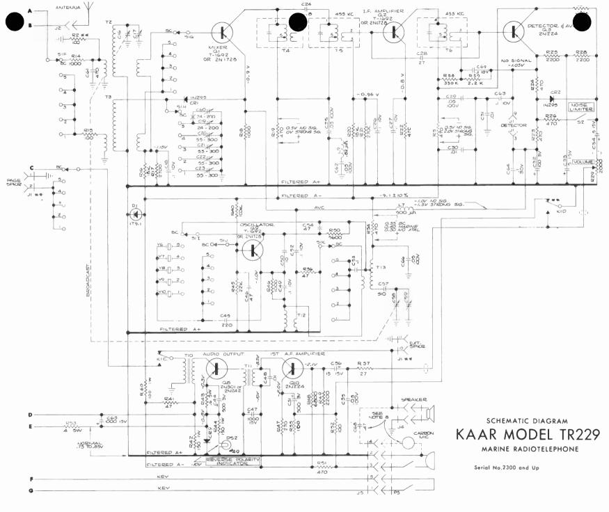
Fig. 3. Schematic of Kaar Marine Unit.
