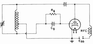
Fig. 12. Shunt-fed Hartley oscillator.
