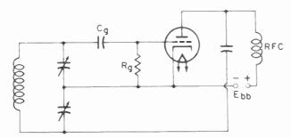
Fig. 14. Shunt-fed Colpitts oscillator.
