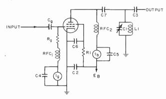
Fig. 3. Shunt-fed Class-C stage.
