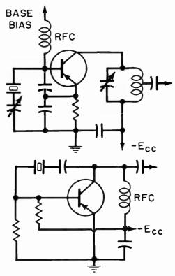
Fig. 11. Transistor crystal oscillators.
