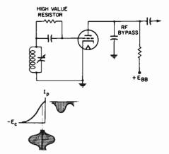
Fig. 12. Basic grid-leak detector circuit.
