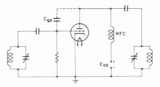
Fig. 16. TPTG oscillator with shunt-fed plate.
