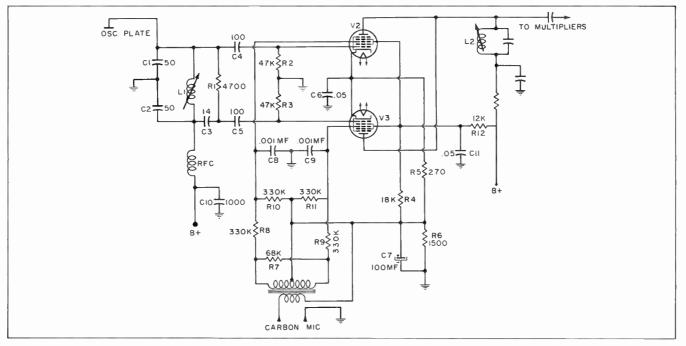
Fig. 5. Typical modern balanced modulator circuit.
