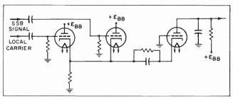
Fig. 7. Fundamental circuit of the Crosby product detector.
