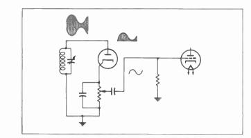
Fig. 10. Diode detector and coupling network to audio amplifier.
