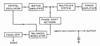
Fig. 4. Block diagram of a basic phase-modulation system.
