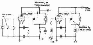
Fig. 4. Oscillator-multiplier adjustments.
