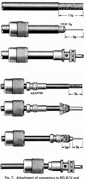
Fig. 7. Attachment of connectors to RG-8/U and RG-58/U cable. (Courtesy RCA)
