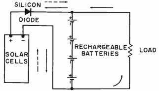
Fig. 8. Solar power supply circuit hook-up.
