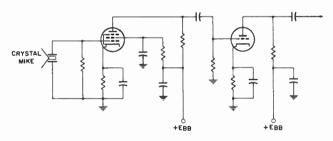
Fig. 17. Crystal microphone in two-stage amplifier.
