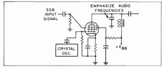
Fig. 6. Simplified product detector circuit.
