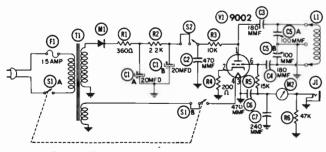
Fig. 6. Circuit of the Millen grid-dip oscillator.
