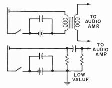
Fig. 2. Carbon microphone circuits.
