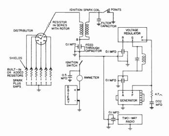
Fig. 10. Noise suppression in vehicle electrical system.
