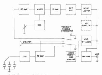
Fig. 1. Functional-block diagram of a Citizens band radio.
