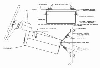
Fig. 4. Mounting the communicator.
