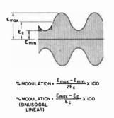
Fig. 12. RF envelope produced with 50% modulation.
