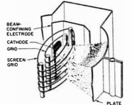
Fig. 10. Basic construction of a beam-power tube.
