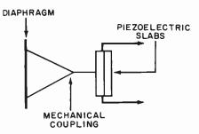
Fig. 3. Construction of a crystal or ceramic microphone.
