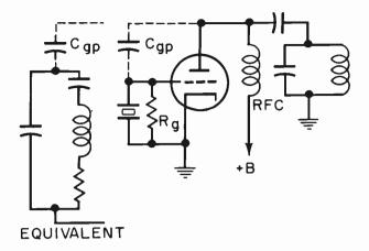
Fig. 6. Triode crystal oscillator and crystal equivalent.
