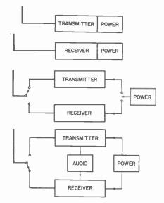
Fig. 3. Basic receiver and transmitter arrangements.
