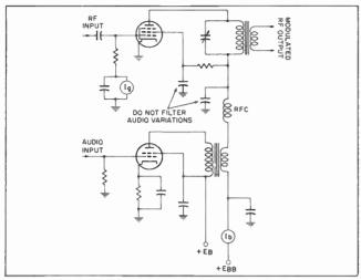
Fig. 8. Simplified plate-modulation circuit.
