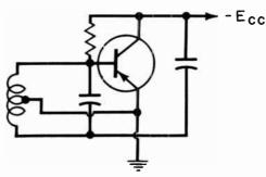
Fig. 10. Transistor Hartley oscillator.
