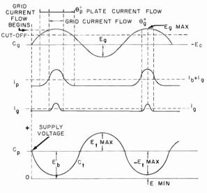
Fig. 4. Class-C waveforms.
