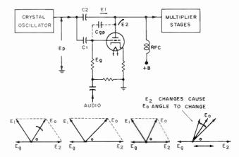
Fig. 6. Vector analysis of a narrow-band phase modulator.
