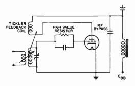
Fig. 13. Basic regenerative detector circuit.
