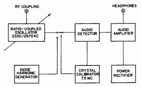
Fig. 15. Functional plan of Lampkin frequency meter.
