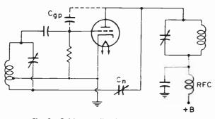
Fig. 9. Grid-neutralization triode RF stage.
