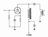
Fig. 16. Coupling to a high-impedance speaker.
