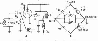
Fig. 7. Plate neutralization of a triode.
