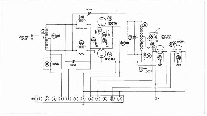
Fig. 9. Schematic of Gates power amplifier.
