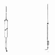
Fig. 4. Coaxial skirt antennas.
