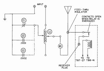
Fig. 10. Antenna coupling network for Gates transmitter.
