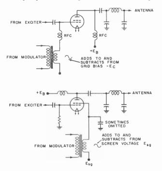
Fig. 3. Other basic AM modulation methods.
