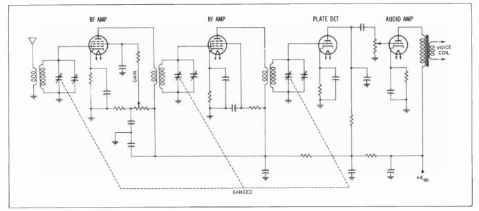
Fig. 6. Tuned RF receiver.
