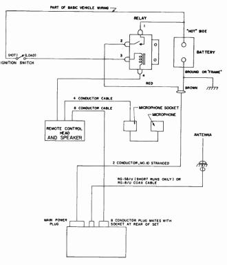
Fig. 10. Aerotron remote-control installation plan.
