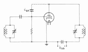
Fig. 15. TPTG oscillator with series-fed plate.
