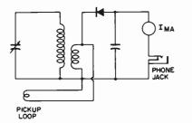
Fig. 3. Absorption wavemeter with pickup loop and phone jack.
