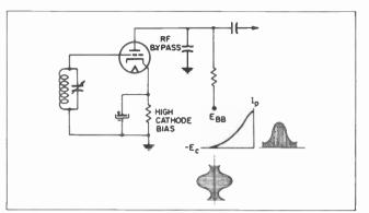
Fig. 11. Basic plate detector circuit.
