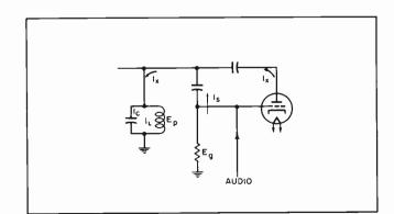
Fig. 3. Basic capacitive-reactance tube circuit.
