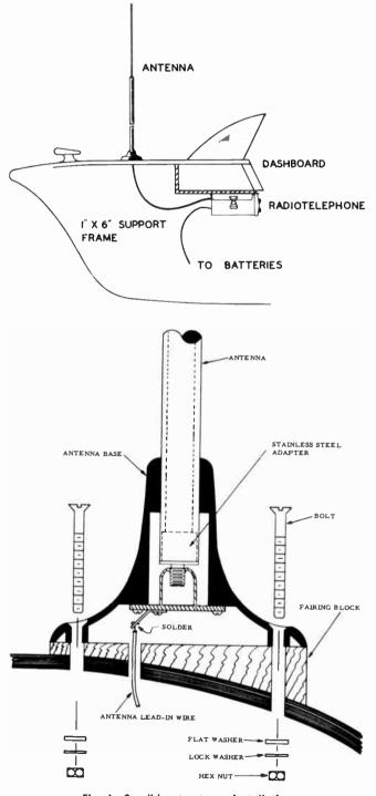
Fig. 6. Small-boat antenna installation.
