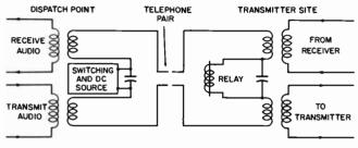
Fig. 13. Basic remote control method.
