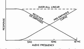
Fig. 8. Over-all frequency response made linear by de-emphasis in the receiver.
