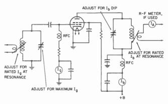
Fig. 1. A metered Class-C amplifier.
