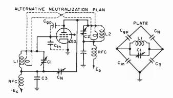
Fig. 8. Neutralization of a screen grid Class-C amplifier.
