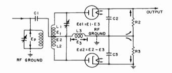
Fig. 8. Conventional phase discriminator circuit.
