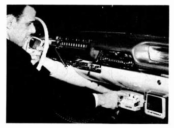
Fig. 2. Two-way radio control box and speaker. (Courtesy Motorola, Inc.)
