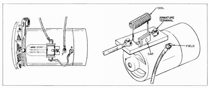
Fig. 11. Noise suppression at the generator.
