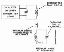
Fig. 1. Principle of the absorption wavemeter.
