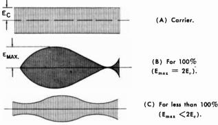
Fig. 20. Envelope check of modulation.
