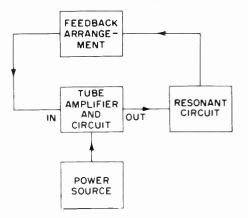
Fig. 13. Block diagram of a basic oscillator.
