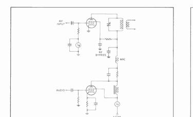
Fig. 10. Basic circuit for Heising plate modulation.
