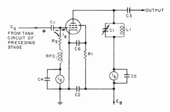
Fig. 2. Series-fed Class-C stage.
