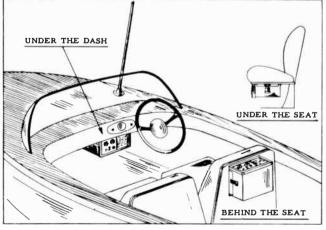
Fig. 5. Raytheon small-boat radio and typical mounting position.
