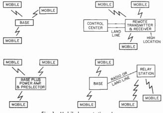
Fig. 1. Mobile base station plans.
