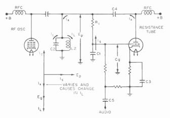
Fig. 2. Simplified schematic of a basic reactance-tube circuit.
