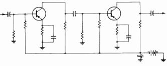
Fig. 18. Transistor two-stage audio amplifier.
