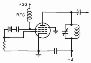
Fig. 8. Pentode crystal oscillator.
