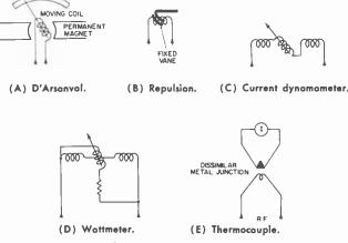
Fig. 11. Basic meter movements.
