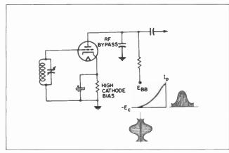
Fig. 12. Basic plate detector circuit.
