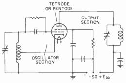
Fig. 4. Basic electron-coupled oscillator (ECO).
