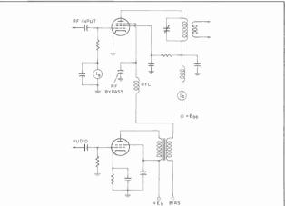
Fig. 11. Circuit designed for suppressor-grid modulation.
