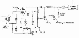
Fig. 5. Power amplifier tuning.
