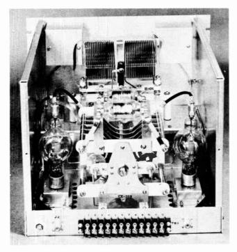
Fig. 8. Final power amplifier of Gates 500-watt transmitter.
