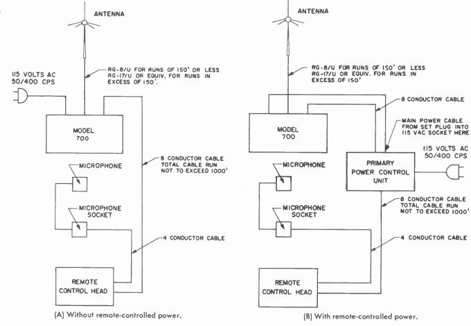
Fig. 12. Telephone-line system for remote control operation.
