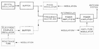
Fig. 1. Functional plan of typical transmitter.
