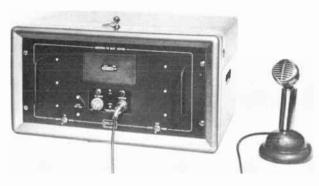
Fig. 6. Aerotron 100-watt base station.
