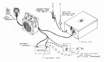
Fig. 2. Basic interconnections of mobile two-way radio components.
