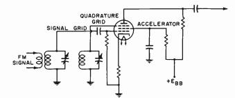
Fig. 10. Basic circuit for a gated-beam detector.
