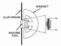
Fig. 4. Basic construction of a dynamic microphone.
