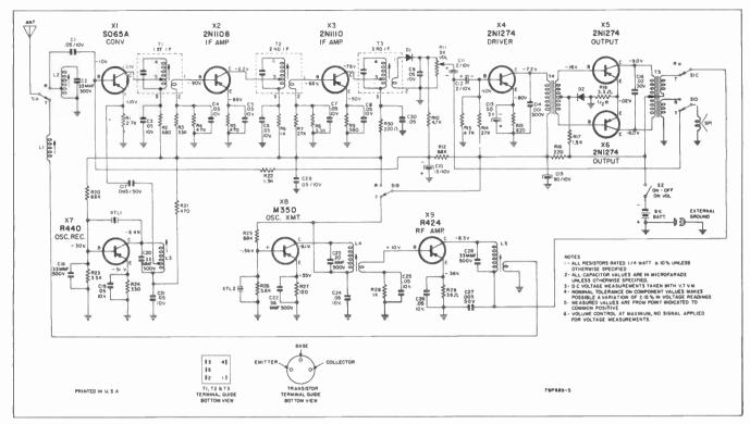
Fig. 5. Webcor hand-held all-transistor CB unit.
