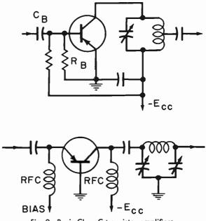
Fig. 9. Basic Class-C transistor amplifiers.
