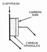
Fig. 1. Basic construction of a carbon microphone.
