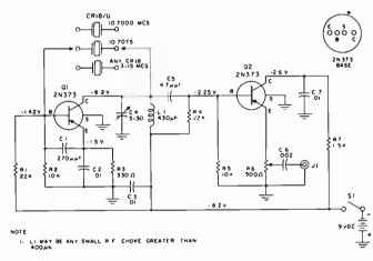
Fig. 3. Receiver alignment test oscillator.
