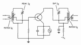
Fig. 7. Tuning Class-C transistor amplifier.
