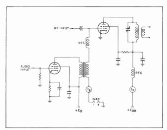
Fig. 9. Simplified grid-modulation system.
