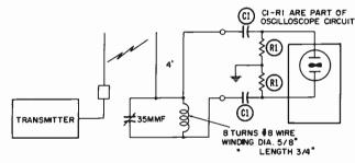
Fig. 19. Simple modulation-envelope check method.
