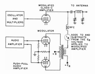
Fig. 1. Diagram of a basic plate modulation system.
