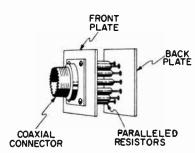
Fig. 10. Home-constructed dummy load.
