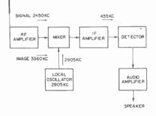
Fig. 7. Functional block diagram of a superheterodyne receiver.
