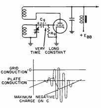
Fig. 3. Basic superregenerative detector, and an analysis of grid and plate currents.
