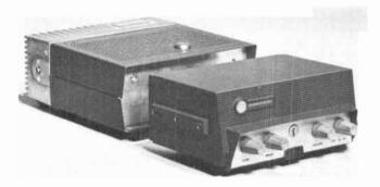
Fig. 8. General Electric transistorized mobile station.
