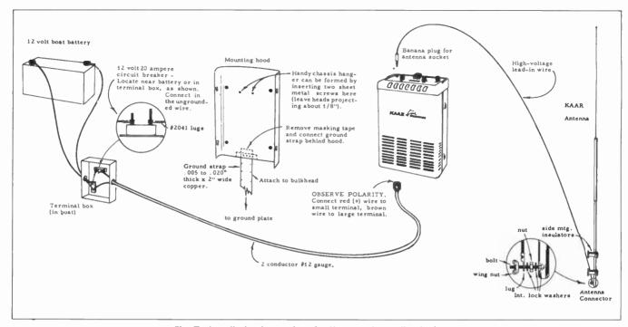
Fig. 7. Installation instructions for Kaar marine radiotelephone.
