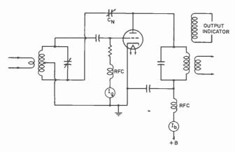
Fig. 3. Triode Class-C amplifiers must be neutralized.
