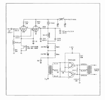
Fig. 6. Modulator and circuits for radiomarine transmitter.
