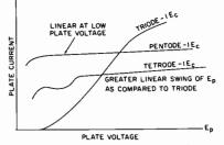
Fig. 9. Characteristics of triode, tetrode, and pentode tubes.
