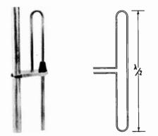
Fig. 7. Wide-band antenna styles.
