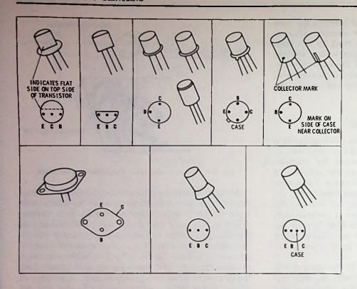
Fig. 14-5. Basing diagrams for a number of popular transistors found in transistor radios.
