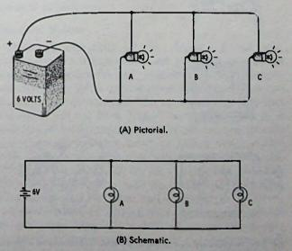
Fig. 2-9. Lamps connected in parallel across a bettery.
