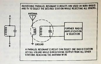
Fig. 14-11. Parallel-resonant circuit and its use to select the signal of a radio station.
