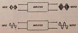
Fig. 8-1. Simple ampiflers, showing relation of output to input.
