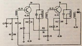
Fig. 11-3. Same circuit as Fig. 11-1, but with reversed supply polarity.
