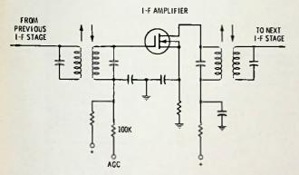
Fig. 16-12. I-f amplifier using MOSFET transistor.
