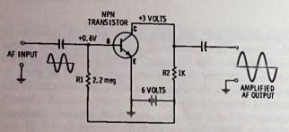
Fig. 8-2. Audio amplifier circuit.
