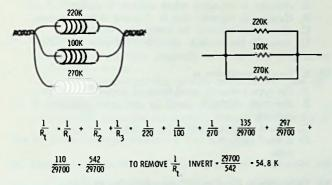
Fig. 2-17. Calculating value of more than two unequal resistors in parallel.
