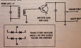
Fig. 6-4. Transistor used as diode decrector.
