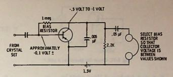
Fig. 8-15. Shunt-feed circuit for crystal headphones (may be used with other phones, too).
