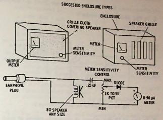
Fig. 12-14. Combination test speaker and output meter with sensitivity control.
