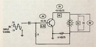
Fig. 8-6. Adding ac signal voltage to the circuit of Fig. 8-5.
