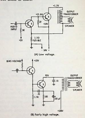
Fig. 12-12, Single-ended output stages.
