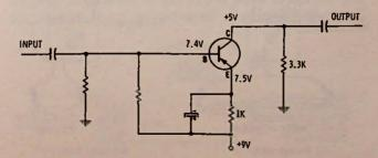
Fig. 9-6. Transistor audio circuit, showing voltage readings to ground.
