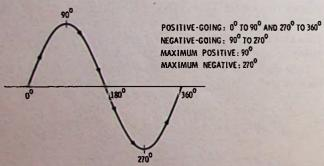
Fig. 7-3. Sine wave showing degree check points.
