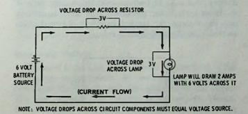
Fig. 1-19. Using Ohm's law to calculate size of resistor.
