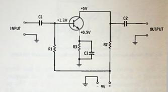
Fig. 8-8. Transistor amplifier stabilized by emitter resistor.
