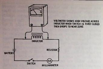
Fig. 14-9. Demonstration circuit to show voltage across inductor as do voltage is first applied.
