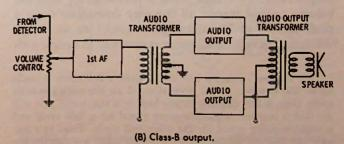
Fig. 7-1. Block diagrams of audio amplifiers.
