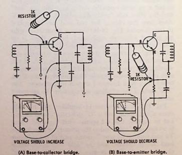
Fig. 14-3. Using a TK resistor to check dc circuits of a transistor stage.
