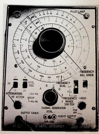
Fig. 9-16. Crystal-controlled signal generator.
