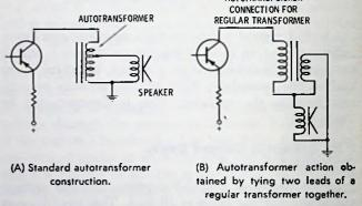
Fig. 3-9. Circuits using autotransformers.
