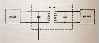
Fig. 5-3. I-f amplifier circuit for amplifiers using high-impedance inpo
