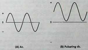
Fig. 3-7. Ac and pulsating dc can both operate a transformer.
