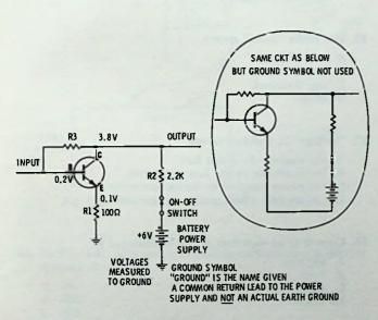
Fig. 1-26. Transistor circuit with voltages to ground indicated.
