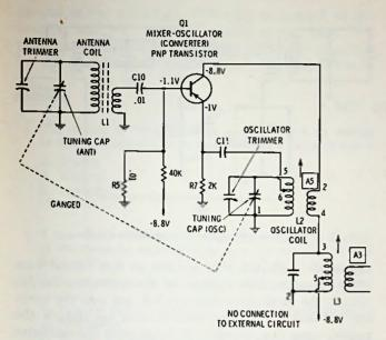
Fig. 10-2. Mixer-oscillator (converter) circuit of a-m broadcast radio.
