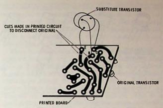
Fig. 14-4. Temporary substitution of transistor on circuit board.
