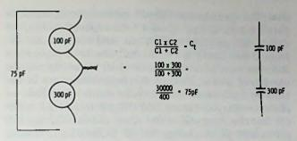
Fig. 2-8. Capacitors of different values in series.
