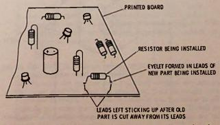
Fig. 15-6. Installing a new resistor from top of printed-circuit board.
