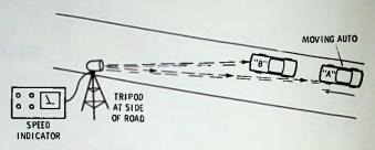
Fig. 1-2. Radar used to check speed of traffic.
