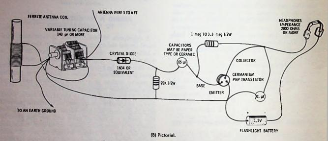
Fig. 8-12. Crystal radio with a one-transistor audio amplifier.
