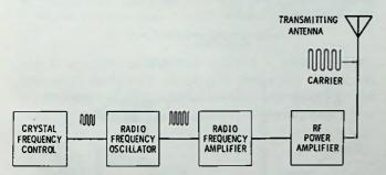
Fig. 1-8. Block diagram of a radio transmitter.
