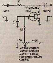
Fig. 16-9. Remote volume control circuit.
