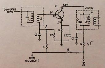
Fig. 11-9. I-f amplifier circuit for Questions 6 through 10.
