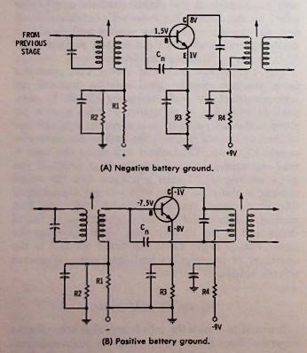
Fig. 13-7. Two fm i-f circuits identical except for ground polarity.
