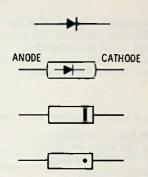
Fig. 6-5. Diodes are marked in various ways to indicate polarity. Usually they are marked at the cathode end.
