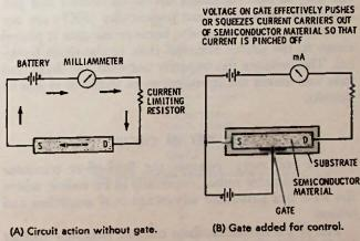
Fig. 16-1. Simple field-offect transistor.
