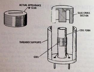
Fig. 5-2. Construction of an adjustable coil in which the tuning slug also serves as a coil shield.
