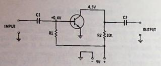
Fig. 8-7. Transistor audio amplifler.
