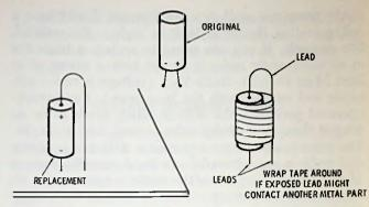
Fig. 15-7. A part with a lead at each end replac<mark>ing a part with both</mark> leads at one end.
