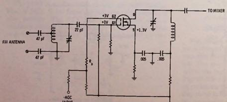
Fig. 16-11. Rf amplifier in fm receiver, using dual-gate MOSFET n-channel transistor.
