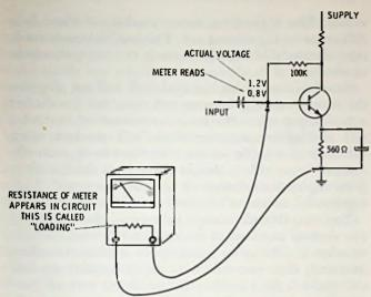
Fig. 9-5. Effect of meter resistance on a voltage measurement, Current through a 100K resistor reduces actual voltage of 1.2V to 0.8V on the 20,000 ohms-per-volt meter.
