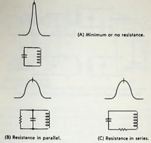
Fig. 14-13. Resonance curves, showing effect of series or parallel resistance.
