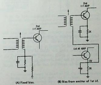
Fig. 11-5. Biasing arrangements for 2nd i-f amplifier.
