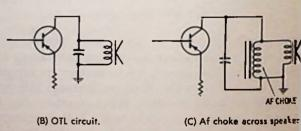
Fig. 7-7. Some class-A audio output stages used in auto radios.
