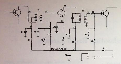
Fig. 14-2, "Hot" and "cold" signal circuits in a transistor amplifier.
