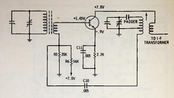
Fig. 10-4. Variation of mixer-oscillator circuit.
