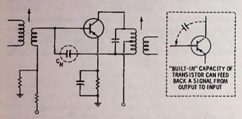
Fig. 11-6. Neutralized i-f stage.
