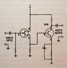
(A) Circuit for npn transistor.
