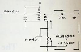
Fig. 6-3. Variation of detector circuit.
