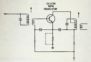
Fig. 11-8. Silicon transistor circuit showing some variations that may not be possible with germanium transistors.
