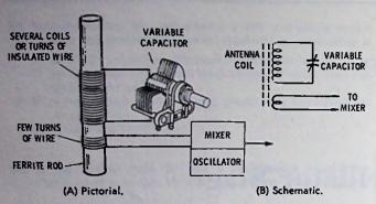
Fig. 4-2. Common method of tuning an antenna coil.
