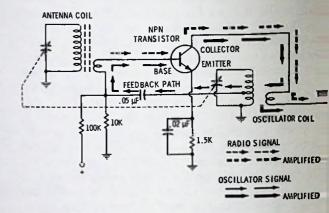
Fig. 4-6. Circuit of transistor mixer oscillator. Note different manne drawing antenna coil, which allows for cleaner schematic layout.
