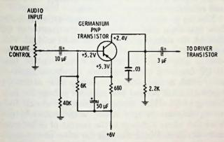
Fig. 12-2. RC-coupled audio stage for additional audio gain.
