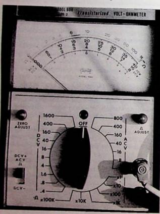
Fig. 9-15. Transistorized volt-ohmmeter.
