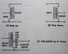
Fig. 3-10. Autotransformer connections.
