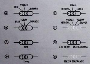
Fig. 2-23. Resistor coding for Questions 35 through 42.
