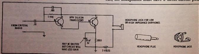
Fig. 8-13. A two-transistor audio amplifier.
