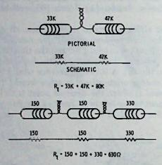
Fig. 2-14. Resistors in series provide total resistance R<sub>1</sub> equal to the sum of the individual resistances.
