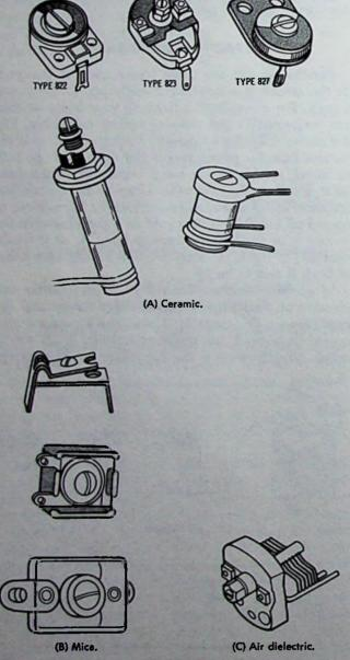
Fig. 2-10. Trimmers are used to adjust the initial capacitance of a circuit, or to "tune" it.
