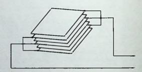
Fig. 2-11. "Stacking" the plates of a capacitor increases the capacity.
