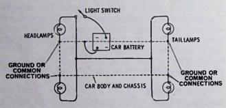
Fig. 2-5. Simplified diagram of an automobile lighting system.
