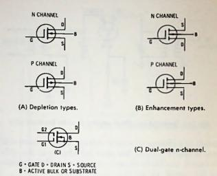
Fig. 16-10. Schematic symbols for IGFET and MOSFET transistors.
