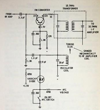
Fig. 13-4. Single transistor serving as both mixer and oscillator.
