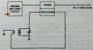
Fig. 4-5. Oscillator is amplifier that "feeds back."
