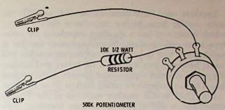
Fig. 12-9. Test circuit for adjusting bias on transistor circuit.
