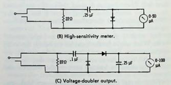
Fig. 11-4. Examples of output-meter circuits.
