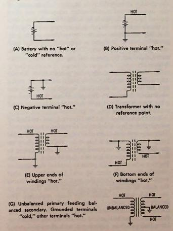
Fig. 14-1. "Hot" and "cold" circuits.
