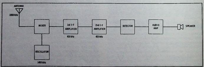
Fig. 1-7. Block diagram of superhet standard broadcast radio.
