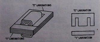
Fig. 2-8. Construction of audio transformer.
