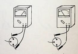
(C) Emitter-to-collector test (see text).
