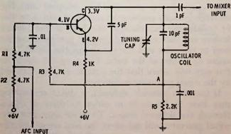
Fig. 13-5. Separate fm oscillator with afc.
