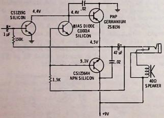
Fig. 12-11. A Motorola "TL" circuit that returns speaker to "hot" side of battery rather than to ground.
