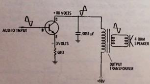
Fig. 7-6. Line-power operated radio using high-voltage transistor.
