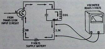
Fig. 1-24. Testing for current by measuring voltage.
