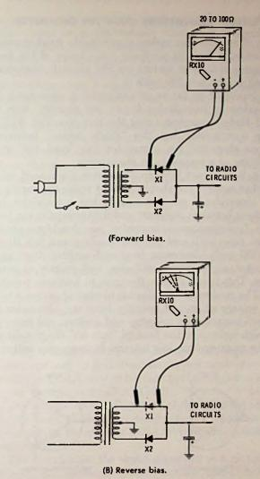
Fig. 9-10. Measurement of rectifier diode may give an inconclusive result (see text).
