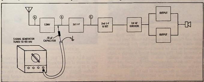
Fig. 9-14. Using a signal generator to locate a defective stage in a radio.
