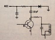
Fig. 13-14. Separate diode used for agc voltage.
