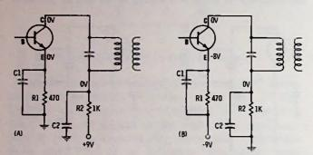
Fig. 15-5. What is the trouble? Is the trouble the same in both circuits?
