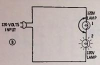
SHORT WHICH MIGHT BE DELIBERATE AND DESIRABLE. LAMP 1 WILL HAVE NO CURRENT THRU IT AND SO WILL NOT BE LIT, BUT LAMP 2 WILL LIGHT TO FULL BRIGHTNESS
