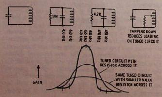
Fig. 5-6. Effect of loading on tuned circuit.
