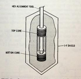
Fig. 13-13. Hex alignment tool reaches bottom core by first passing through top core.
