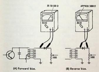
Fig. 9-9. Measuring diodes in-circuit.
