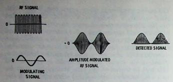
Fig. 1-9. Amplitude modulation is the changing of the rf power output in step with a modulating signal.
