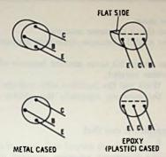
Fig. 8-14. Common basing diagrams for silicon transistors (lead view).
