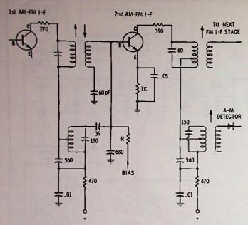
Fig. 13-16. Combination am/fm circuit using capacity matching.
