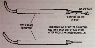
Fig. 13-6, Isolation probes used with vom.
