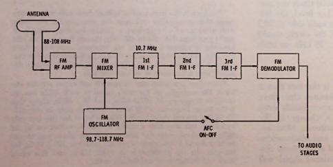
Fig. 13-2. Block diagram of fm radio.
