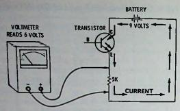
Fig. 1-23. How much current is flowing in this circuit?
