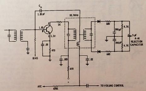
Fig. 13-9. Fm demodulator. This is a ratio detector.
