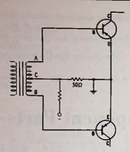
Fig. 15-1. Circuit suitable for testing with ohmmeter.
