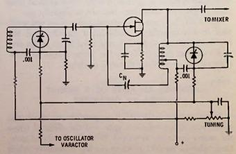
Fig. 16-17. An fm rf stage tuned by varactors.
