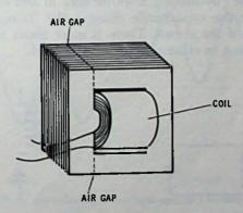
Fig. 3-2, tron-core inductor with a "closed" core. Air gap prevents core saturation.
