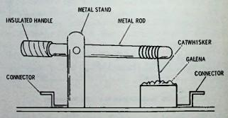
Fig. 1-12. Crystal and catwhisker detector unit used in early days of radio and still available for the experimenter.
