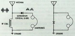
(A) Diode in series, passing positive excursions of signal. (B) Diode in parallel; positive excursions operate headphones.
