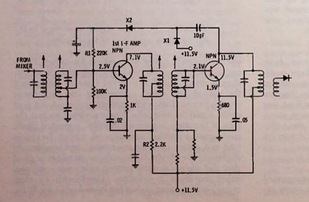
Fig. 11-7. I-f amplifier using forward agc.
