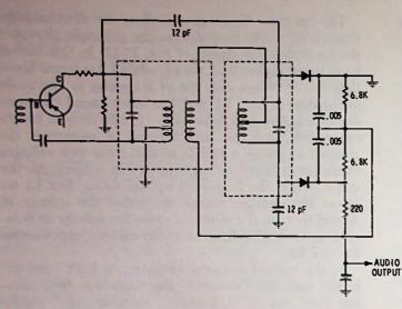
Fig. 13-10. Discriminator circuit. Note that diodes face in the same direction.
