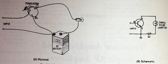
Fig. 8-3. Pilot lamp does not light in this circuit because transistor is "turned off."
