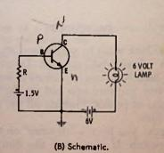
Fig. 8-4. Bias battery "turns on" the transistor, causing lamp to light.
