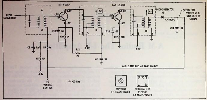
Fig. 11-1. Schematic of i-f amplifier for broadcast radio.
