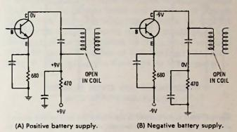
Fig. 15-4. Checking for an open coil, using voltage measurements.
