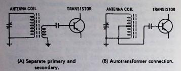
Fig. 3-11. Antenna coil (transformer) circuit in a typical transistor radio.
