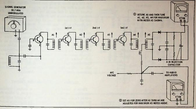
Fig. 13-12. Setting up (alignment) of fm radio that uses ratio detector. Keep signal generator output low.
