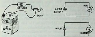
Fig. 1-18, Resistance in a circuit reduces current.
