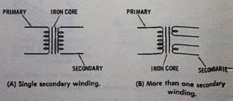
Fig. 3-4. Schematic symbols of audio or power transformer.
