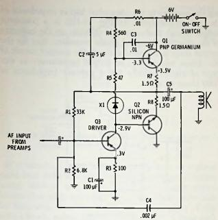
Fig. 12-8. "TL" audio amplifier. Note that one npn and one pnp are used as output transistors.
