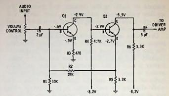
Fig. 12-4. Direct-coupled 2-stage audio preamplifier circuit.
