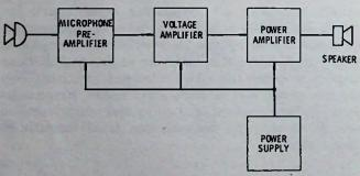
Fig. 1-6. A more detailed "black box" diagram is called a block diagram.
