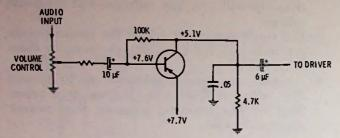
Fig. 12-3. Simple preamplifier circuit.
