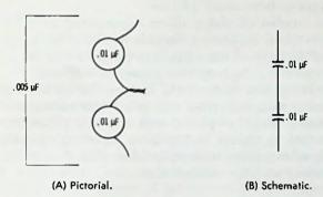
Fig. 2-7. Equal-sized capacitors in series.
