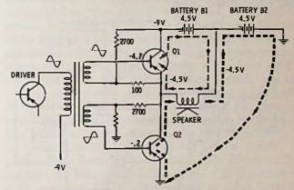
Fig. 12-5. OTL circuit using a center-tapped battery supply.
