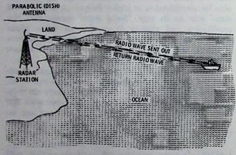
Fig. 1-1. Radar finds a ship and determines how far away it is.
