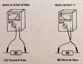
Fig. 9-8. Checking diodes with a vom. Polarity marks are for voltage measurement. Polarity of ohmmeter leads is normally the reverse of this (see text).
