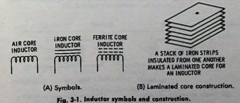
An inductor may also be called either a coil or a choke.
