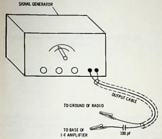
Fig. 13-8. Signal generator has 100-pF isolation capacitor in series with output lead.
