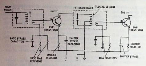
Fig. 5-5. Partial i-f amplifier circuit in an abroadcast radio.
