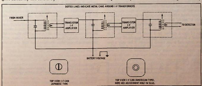
Fig. 5-1. Combination circuit and block diagram of an i-f amplifler.
