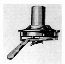
Fig. 14-1. Edison Model H reproducer had sapphire point with a tip radius of .0047 designed to play the new 4-minute records.
