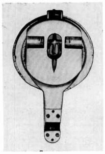
Fig. 8-3. Edison's improved reproducer had a cork-stiffened diaphragm and spring-loaded weight.
