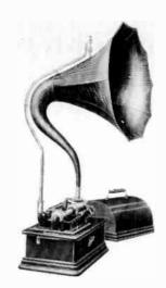
Edison "Home" phonograph of 1911 had an open-ended mandrel. The machine played both two- or four-minute records by means of a turn-over Type O reproducer. Proper gear pitch was selected by a manual gear changer. (Clark-Welch Collection.)
