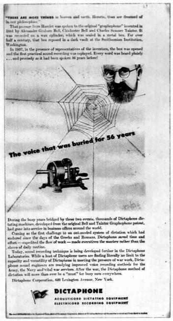
Fig. 3-2. The original "Graphophone"—almost identical to the \$15.00 Edison tinfoil phonograph, but with wax in the grooves of the metal cylinder to receive the recording.
