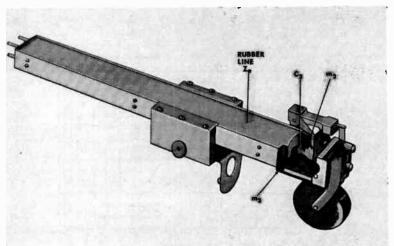
Fig. 10. This figure shows an electromagnetic recorder complete except for the bottom of the case.
