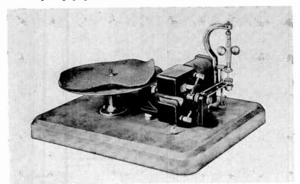
Fig. 10-2. Berliner disc Gramophone operated by a direct-current motor. Speed was controlled by a two-ball governor, 1896. (Courtesy of Smithsonian Institution.)
