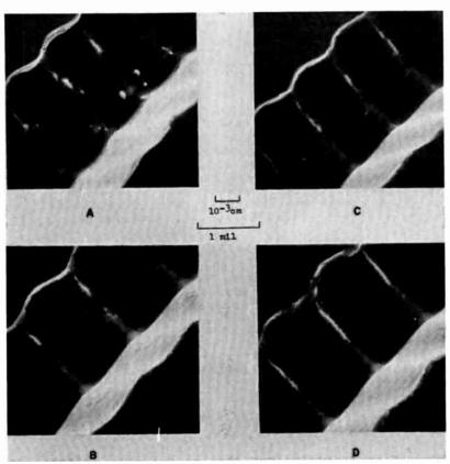
Fig. 30-9. These photos show groove wear caused by four different pickups following 50 plays. Photo A shows the wear produced by a spherical .7 mil stylus tracking at 5 grams; B shows the effect of a  $2\times.7$  mil elliptical stylus at 1.5 grams; C, a  $2\times.9$  mil elliptical stylus at 1.5 grams; and D, a .7 mil spherical stylus at 1.5 grams. (Courtesy of RCA Laboratories.)
