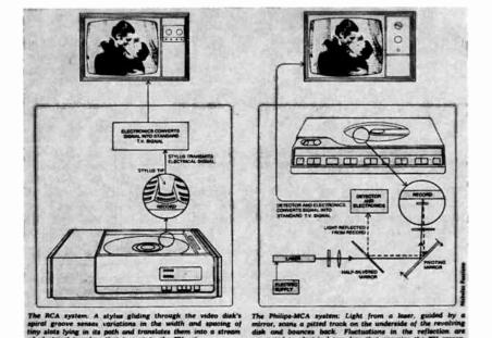
Fig. 30-10. Two proposed video-disc systems for use in the U.S. (Courtesy of the New York Times Magazine.)14
