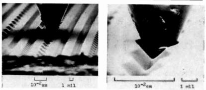
Fig. 30-7. Scanning electron microscope images of a diamond playback stylus in a groove of a vinyl record carrying vertical modulation. (Courtesy of RCA Laboratories.)
