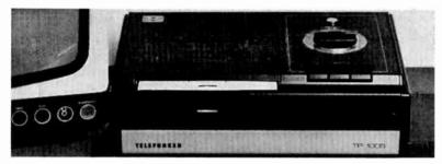
Fig. 30-3. The TED Videodisk player Model TP 1005. (Photo courtesy of Telefunken/Teldec.)
