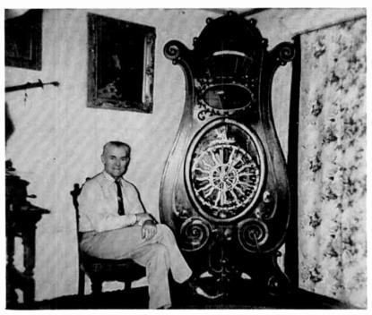
Fig. 9-2. The Multiphone was a monstrous coin-operated "jukebox" and contained 24 cylinders mounted on a large wheel. (Courtesy of C. Y. deKay.)
