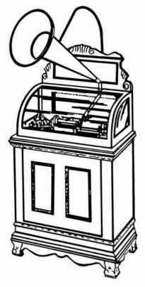
Fig. 9-1. The Edison "M" coin-slot phonograph powered from a storage battery and was usually operated by a nickel.
