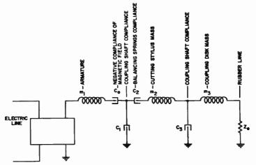
Fig. 12. Equivalent electric circuit of the electromagnetic recorder.
