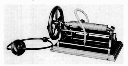
Fig. 3-8. A heavy drive wheel served to stabilize rotation of Tainter's cylinder when rotated by hand. Hearing tubes were used for reproduction. (Courtesy of Smithsonian Institution.)
