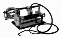
Fig. 4-1. This Tainter Graphophone operated by means of a treadle similar to the early sewing machines. The reproducer is in position and connects to hearing tubes. The recorder (in upright position) may be swung down after reproducer is lifted clear. (Courtesy of Oliver Read collection.)
