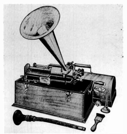
Fig. 5-3. First of several models known as the Edison Home phonograph. It was a spring-motor type and produced sufficient volume to be heard through a 14-inch horn. A shaving knife permitted erasure of sounds for cylinder reuse.
