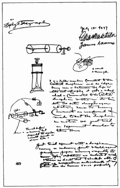
Fig. 2-1. Experiment with diaphragm having an embossing point held against moving paraffin paper. (Courtesy of Edison National Historic Site.)
