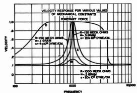
Fig. 9. Velocity response for various values of mechanical constants.
