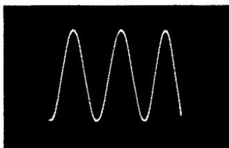
Fig. 4-8. Centered sine-wave pattern.
