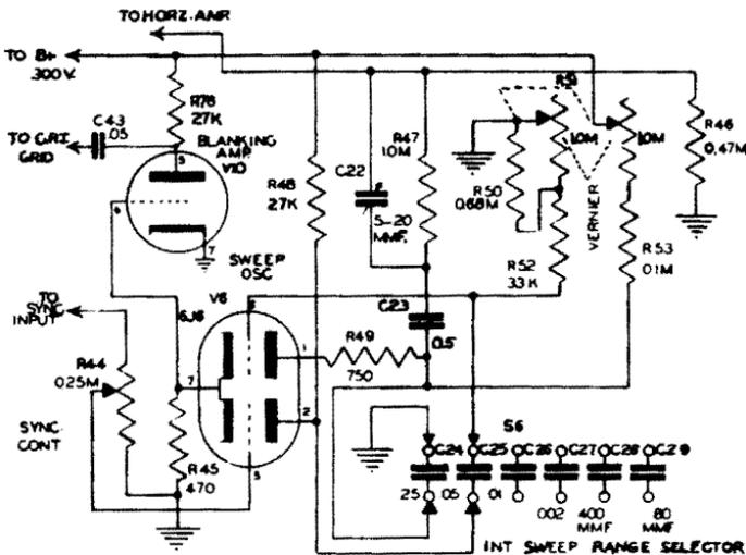
Fig. 1-25. Typical sawtooth (sweep) oscillator and blanking amplifier.
