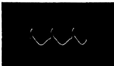
The RC network in the grid of V1 is a filtering and holding configuration. It provides a smooth DC control voltage to the grid, and it also delays passage of sudden input changes. As a result, noise pulses tend to average out and the oscillator is less likely to tear the picture when the noise level is high. Look for open capacitors if appreciable AC is found at the grid of V1.
