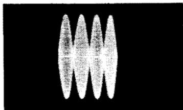
(A) Output waveform from AM generator.
