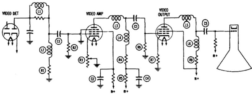
Fig. 3-18. Typical video-amplifier circuit.
