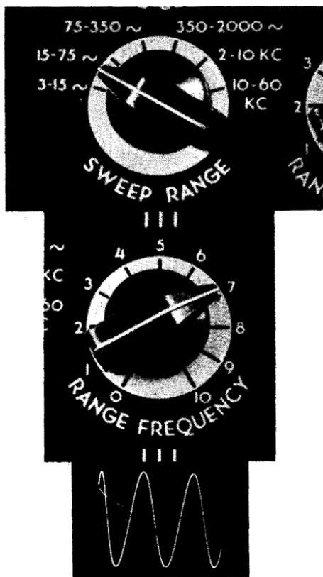
Fig. 1-12. Frequency controls.
