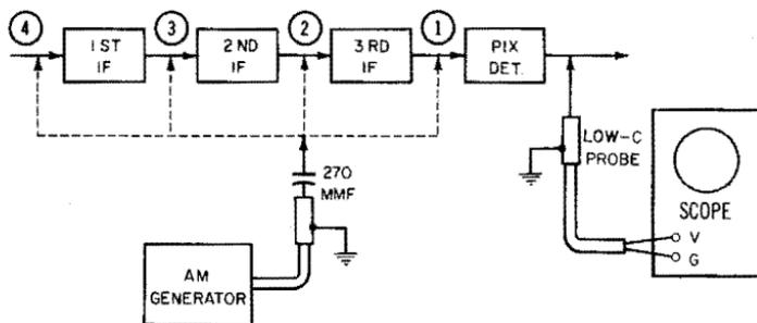
Fig. 3-16. Stage-gain test setup.
