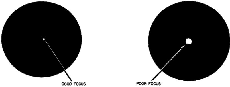
Fig. 1-4. Action of focus control.
