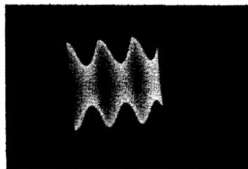
**Fig. 10-7.** Envelope variation at lower percentage modulation.
