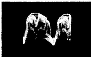
Fig. 4-6. Noise-gate signal applied to point F.
