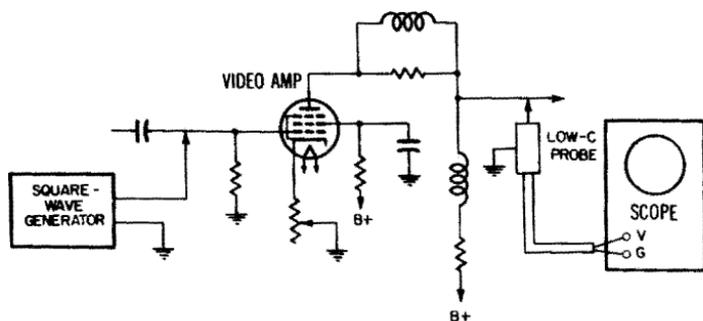
Fig. 2-15. Video amplifier serves as utility wide-band amplifier.
