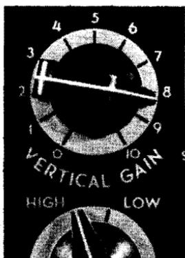
Fig. 1-16. Vertical-gain control effect.
