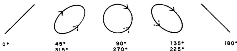
Fig. 11-4. Typical phase-shift patterns.
