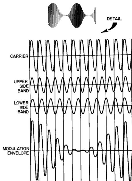
Fig. 2-16. Build-up of a modulated sine wave.
