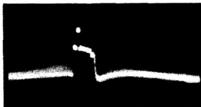
Fig. 3-22. Video signal with white portions compressed.
