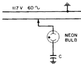
Fig. 2-19. C provides a return circuit.
