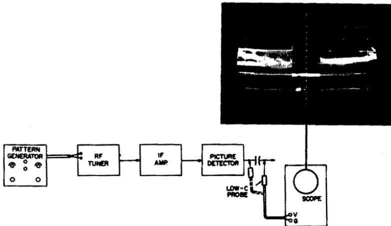
Fig. 3-19. Signal tracing across a coupling capacitor.
