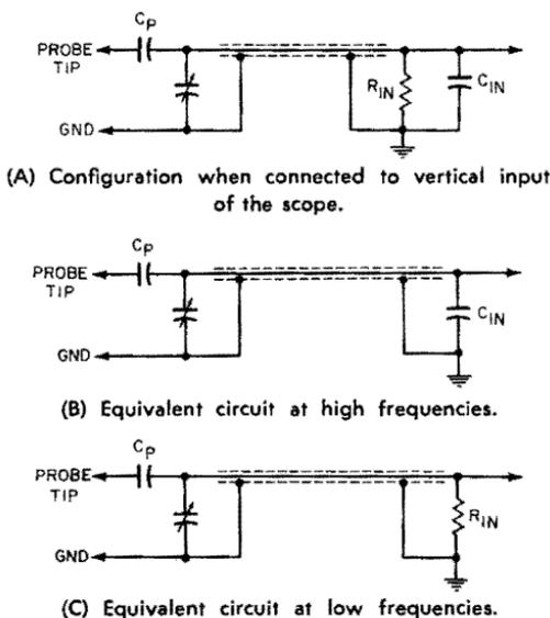
**Fig. 2-10. High-voltage capacitance-divider probe, and its load circuit.**
