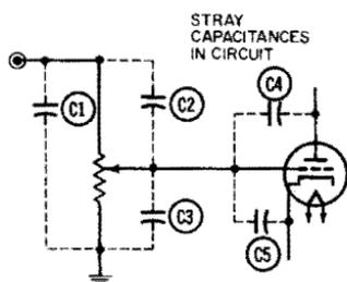
Fig. 1-18. Potentiometer gain control.
