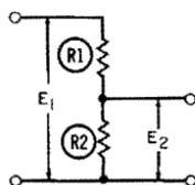
$$E_2 = E_1 \frac{R_2}{R_1 + R_2}$$
