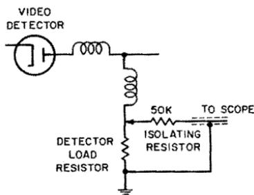
Fig. 2-7. A resistive isolating probe.
