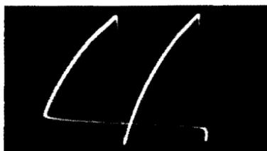
Fig. 5-4. Normal sawtooth waveform from horizontal-oscillator circuit.
