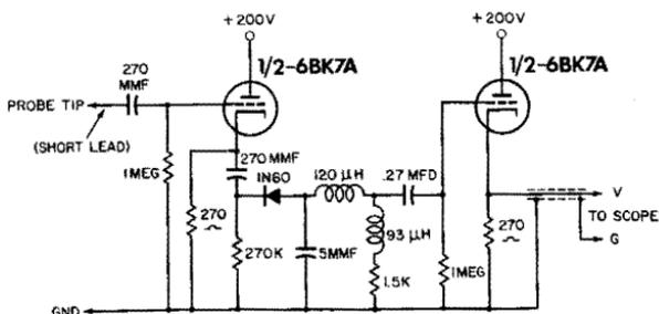
Fig. 3-10. Wide-band demodulator probe.
