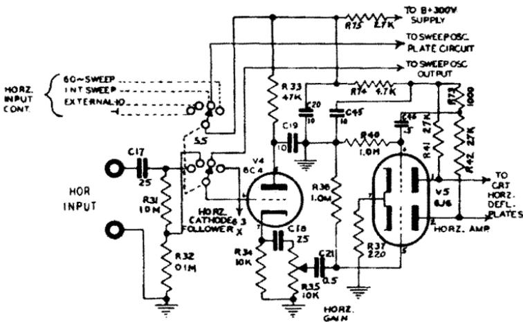
Fig. 1-24. Typical horizontal-amplifier circuit.
