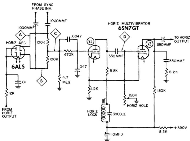
Fig. 5-17. Multivibrator with ringing coil.
