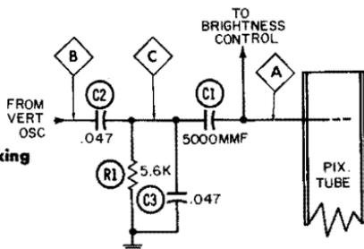
Fig. 7-14. Vertical-retrace blanking circuit.
