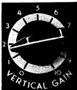
Fig. 1-15. Vertical-gain control incorrectly set.
