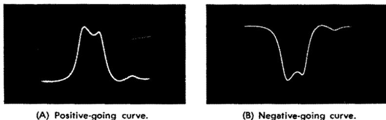
Fig. 2-12. Sweep-alignment curves.
