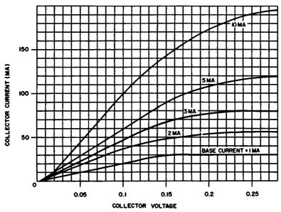
Fig. 10-8. Typical collector saturation characteristics.
