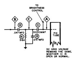
Fig. 6-7 Vertical-retrace blanking circuit.
