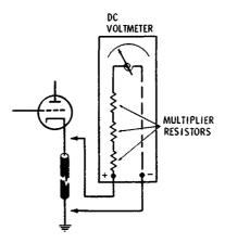
Fig. 10-6. Open cathode resistor causes B+ to appear on cathode.
