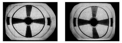
Fig. 5-3. Examples of horizontal nonlinearity.
