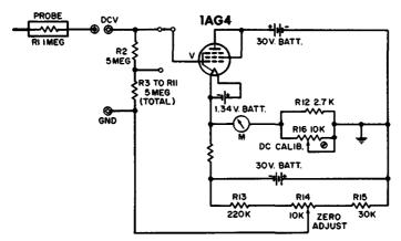
Fig. 1-17. VTVM-adapter configuration.
