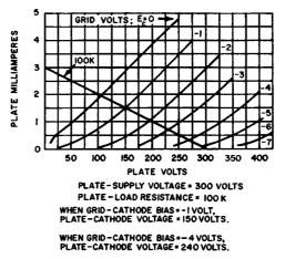
Fig. 9-2. Typical variation of plate voltage with grid bias.
