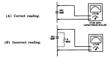
Fig. 4-5. Shunt resistance causes incorrect indication of capacitance value.
