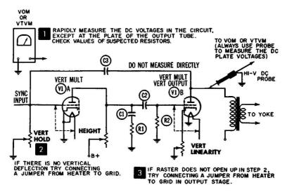
(A) Preliminary tests in the vertical circuitry.
