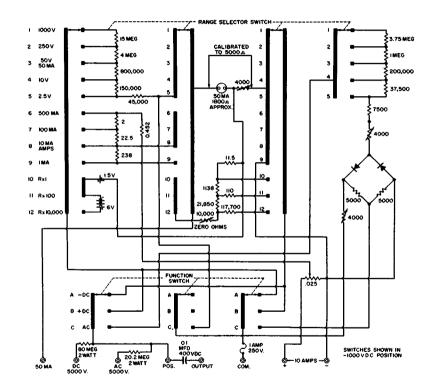
Fig. 1-12. A typical VOM circuit.
