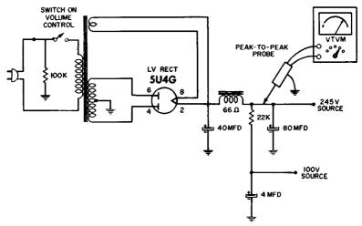
Fig. 8-1. Measurement of ripple voltage.
