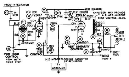
Fig. 6-5. Vertical-drive voltage can be applied from a TV analyzer.
