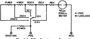
multiplier resistors are switched in series with the meter movement to obtain various full-scale indication values.
