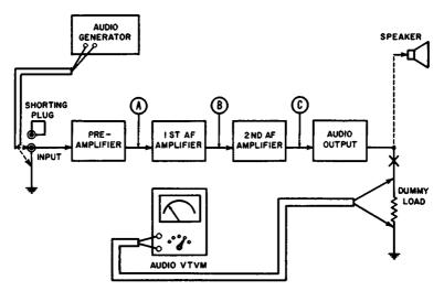
Fig. 9-4. Localizing a noisy amplifier stage.
