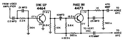
Fig. 3-12. Typical transistorized sync-section of a TV receiver.
