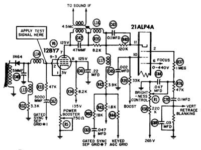
through a small blocking capacitor prior to the sound take-off point, it usually is possible to signal-trace the entire sound section. Offhand, this might seem to be impossible, because the limiter stage normally rejects amplitude modulation. On the other hand, most AM generators have appreciable incidental FM, particularly when set for high-percentage modulation. Incidental FM makes it possible for the generator to do double duty in testing the sound section.
