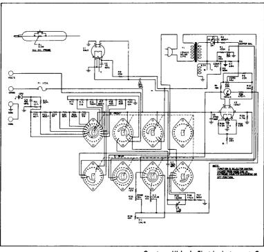
Courtesy Hickock Electric Instrument Co. Fig. 1-18. Circuitry of a typical service-type VTVM.
