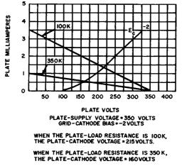
Fig. 9-3. Variation of plate-cathode voltage with load resistance.
