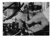
arc or none at all means the horizontal-sweep system is probably defective. (It is assumed that good tubes have been plugged in.) Proceed to the grid circuit of the horizontal-output tube, and measure the negative DC-grid bias there—or better still, check the grid-drive waveform. If drive is normal, the
