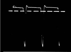
Fig. 3-5. The positiveand negative-peak voltages of stripped sync are widely different.
