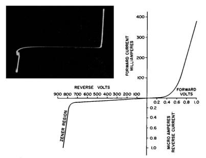
Fig. 1-6. Characteristic of a typical silicon-junction diode.
