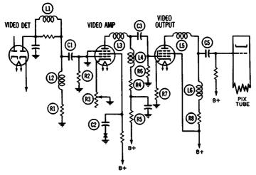
Fig. 2-21. Video-amplifier circuit.
