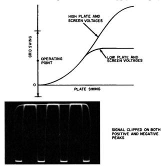
Fig. 7-5. Principle of limiter operation.
