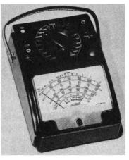
Fig. 1-4. A typical VOM with built-in overload protection.
