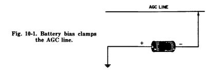
Should the picture and/or sound symptom clear up when the battery is connected, the trouble is in the AGC circuit. Otherwise check the signal circuits, as explained in the previous chapters. Many modern receivers have branched AGC lines to the RF and IF sections (Fig. 10-2). When the RF line is shunted by an AGC-clamp tube, it is good practice to connect two batteries, one to each line. Bias packs often have two
