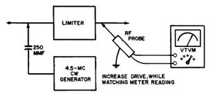
Fig. 7-3. Limiter saturation test.
