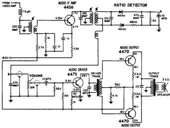
Fig. 7-6. Typical transistorized sound section of a TV receiver
