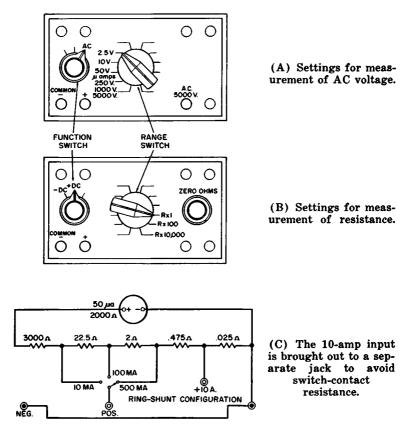
Fig. 1-1. Examples of range- and function-switch settings for a VOM.
