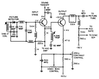
Fig. 2-23. Typical transistorized-video amplifier.
