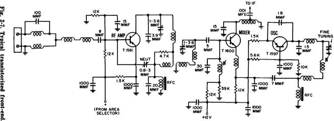
Fig. 2-7. Typical transistorized front-end.
