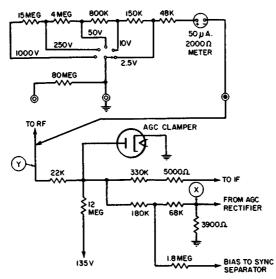
Fig. 10-2. Measuring AGC voltage.
