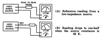
Fig. 3-3. Difference reading with a source resistance.
