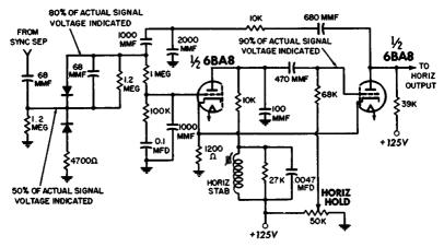
Fig. 4-8. Examples of circut-loading errors in signal-voltage readings.
