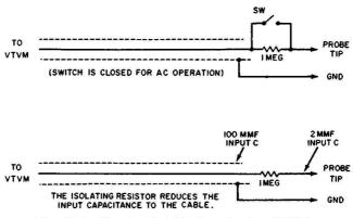
Fig. 11-3. Circuit of AC-DC probe for VTVM.
