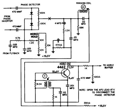
Fig. 4-9. Typical semiconductor AFC and horizontal-oscillator circuit.
