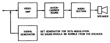
Fig. 7-4. AM rejection test.
