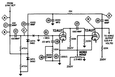
Fig. 4-4. Freewheeling test is made in this circuit by breaking the lead at X and grounding the 1-meg resistor.
