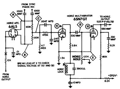
Fig. 4-7. Multivibrator with ringing-coil stabilization.
