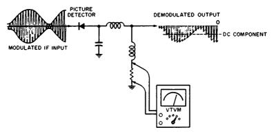
Fig. 2-17. Metering the DC component at the picture-detector output.
