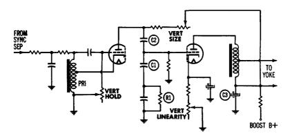
Fig. 6-4. Vertical oscillator and output configuration.
