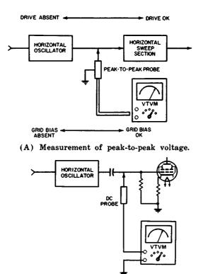
(B) Measurement of signal-developed bias. Fig. 5-1. Two common methods of checking drive voltage.
