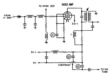
Fig. 2-22. Frequency response being partially controlled by C1, C2, and C3.
