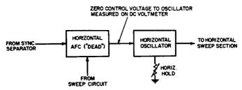
Fig. 4-1. Localization of a dead horizontal-AFC section.
