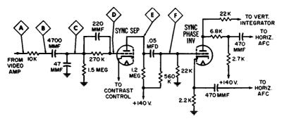
Fig. 3-11. Sync-separator and phase-inverter circuit.
