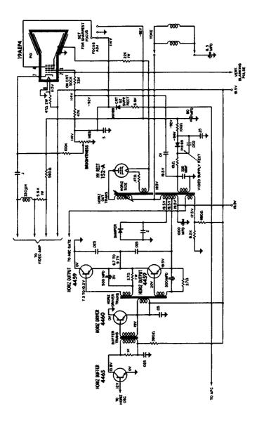
Fig. 5-13. A typical transistorized horizontal-sweep section.
