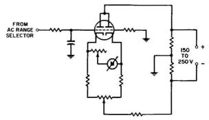
Fig. 11-5. Typical metering measuring circuit.
