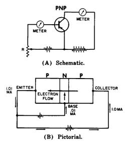
Fig. 2-24. Common-emitter current flow.
