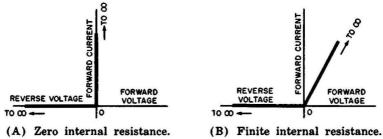
Fig. 1-5. Ideal diode characteristics.
