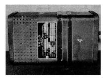
Fig. 2-6. A constant-voltage line transformer.
