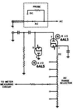
Fig. 11-4. Conversion circuit of AC-DC probe.
