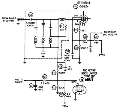
Fig. 10-5. AGC and 1st-IF amplifier circuitry.
