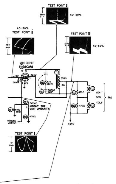
\* DO NOT MEASURE UNLESS 100-TO-1 HIGH-VOLTAGE DC PROBE 15 USED \* # USE LOW-C PROBE TO CONNECT SCOPE TO TEST POINT 3
