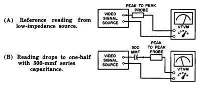
Fig. 3-4. Source reactance reduces voltage indication.
