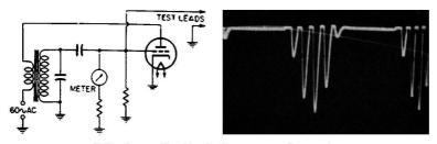
(B) A continuity indicator configuration. Fig. 5-10. Using the flybacker as a capacitance checker.
