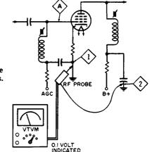
Fig. 2-16. Grounds 1 and 2 are at different 40-mc potentials.
