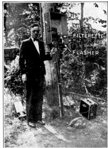
FIG. 65. Checking interference from a traffic flasher.
