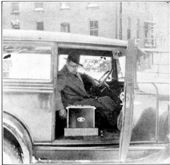
FIG. 99. Installation of Interference Locator in the trouble car of the Public Service Company of New Hampshire.
