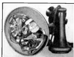
FIG. 25. Installation of Tobe Dial Filterette in the base of a dial telephone.
