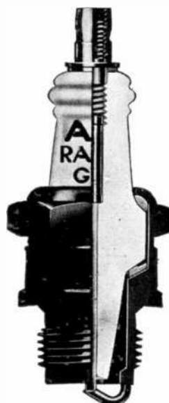
FIG. 106. Cut-away view of an A. C. spark plug showing filtering spark suppressor.
