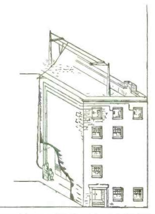
Apartment houses and hotels can have a radio telephone receiver in every apartment. A common aerial on the roof and a common receiving set in the basement with telephone or loud-speaker connections in the apartments—nothing more is required
