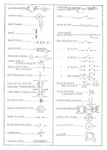
Symbols used in wiring diagrams
