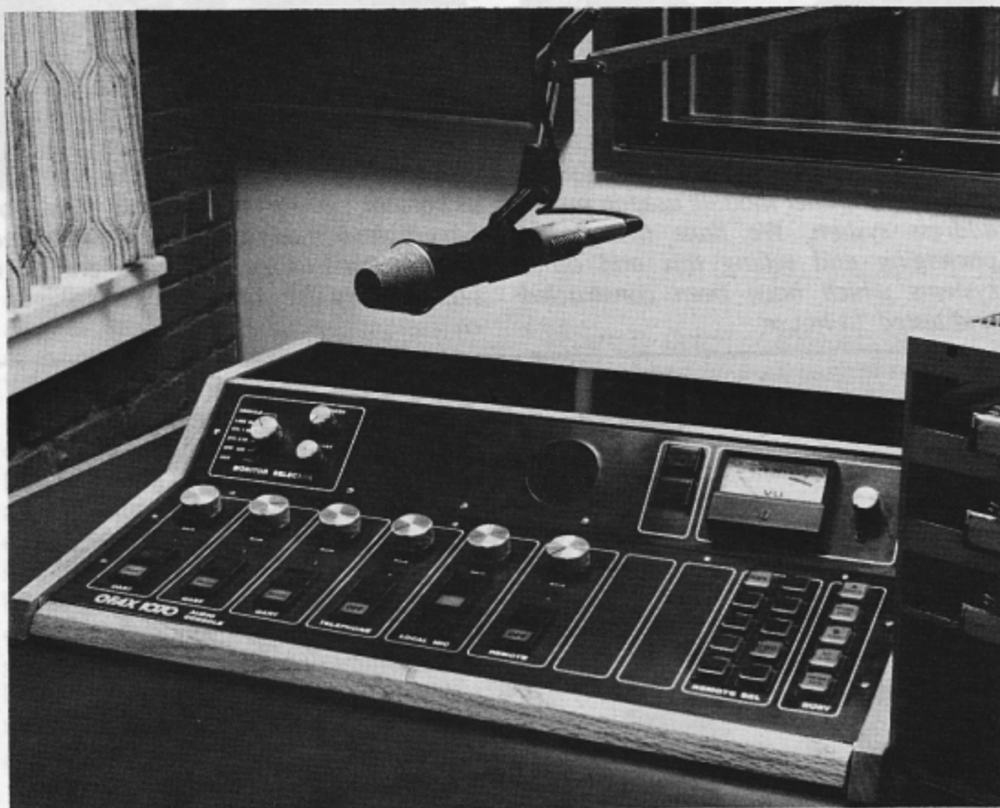
Photo 4: Six-channel mixer used in sports studio. Inputs from left to right are 3 carts, telephone, microphone and remote. On far right, a remote selector and intercom system. This console has channel logic similar to BMX consoles, mainly to incorporate cartridge replay lockout.
