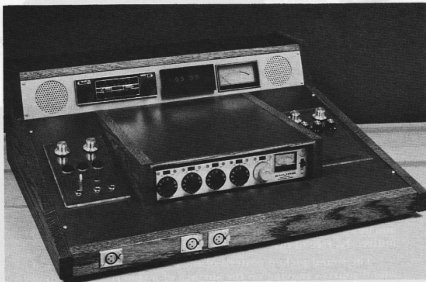
Photo 8: Console designed for remote broadcast cut-ins is complete with built-in UHF talk-back facilities.
