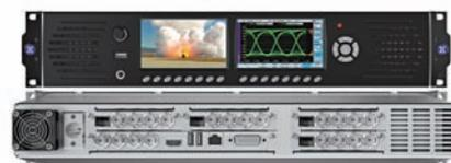
Two 4.3 inch 16:9 aspect ratio screens are located on the front panel of the Rx2000, one assigned to video confidence monitoring and the other to menu viewing and instrumentation. Forward-facing wide-range audio monitor loudspeakers are located left and right of the displays. A quarter-inch stereo audio jack socket and USB-2 port are also on the front panel.
