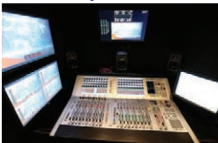
A Studer Vista 1 mixing console from Harman resides in one of the newest OB trucks from Montreal's REC4BOX.
