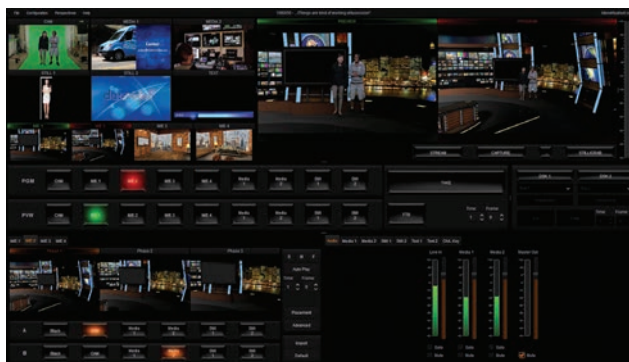
The interface to Datavideo new TVS 1000 virtual production system offers full control over video assets, inputs and outputs.
