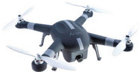
The Aries Blackbird X10 quadcopter has an on-board HD video camera.
