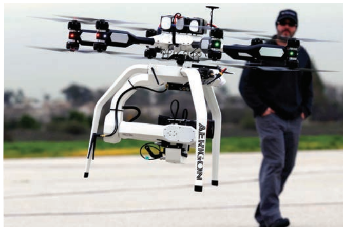
The Aerigon Gimbal features an advanced stabilization system to work with heavy cameras.
