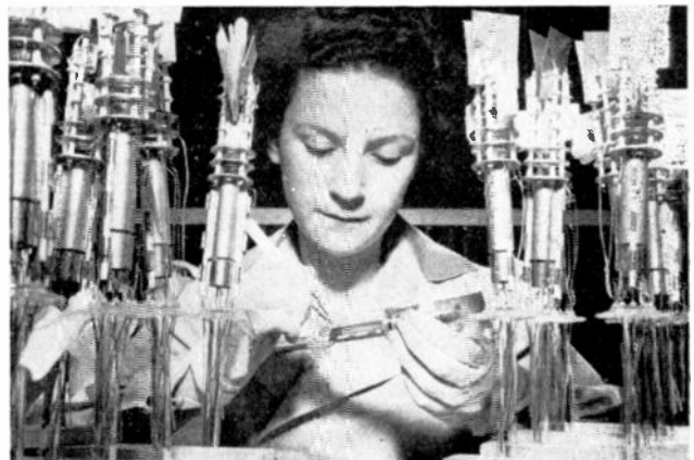
Checking the mount mechanism at Research Enterprises.
