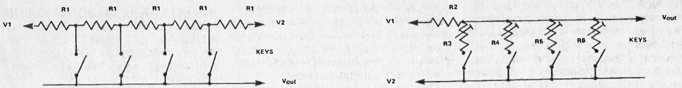
Fig. 1 Two methods of keyboard decoding used in the multiphonic synthesiser
