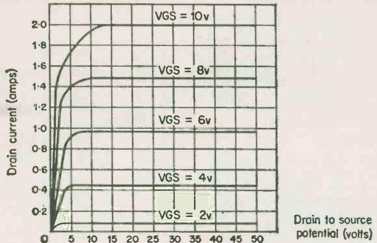
Fig. 3. Typical output characteristic of a VMOS transistor.
