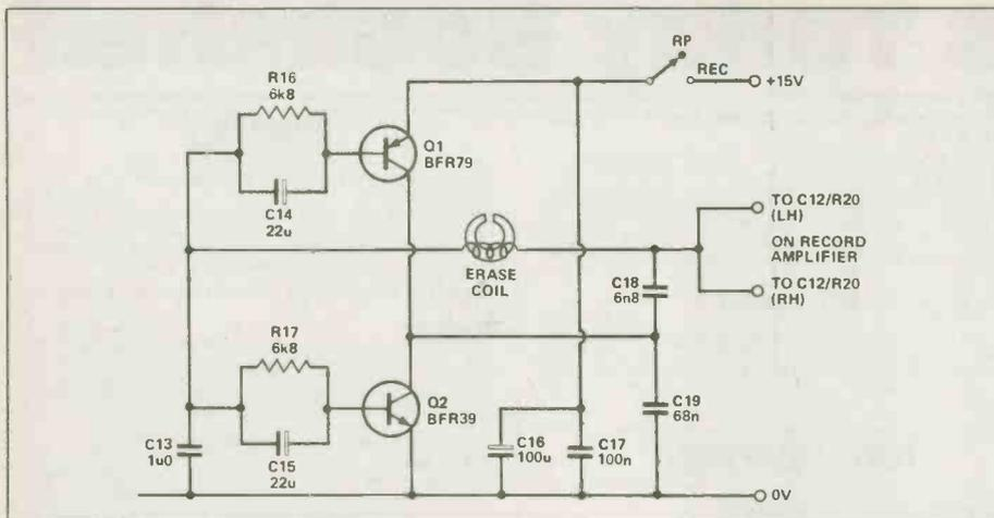
Fig. 15. A cassette recorder bias and erase oscillator.
