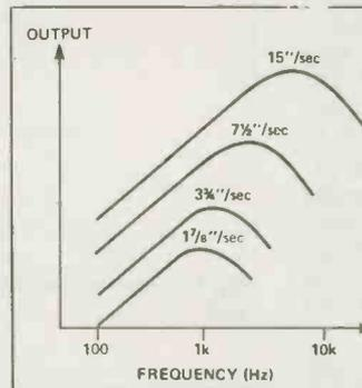
Fig. 7. (left) Output level versus frequency response for different tape speeds.
