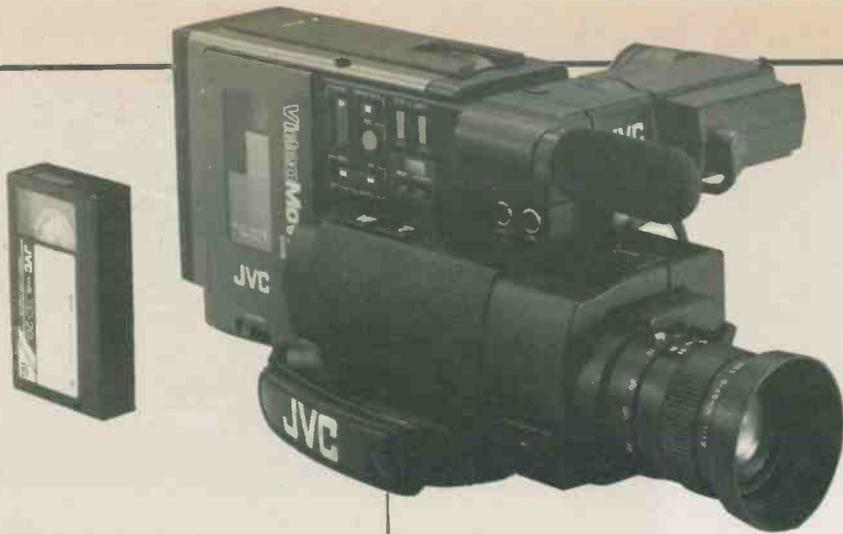
half-inch built-in electronic viewfinder, or alternatively, by fitting the VHS-C into a special cartridge (analogous to the cartridges which permit cassette tapes to be played on 8-track units) the footage can be viewed via standard VHS playback units and a television set. The tape can also be played back through an A/V monitor or (via a built-in RF unit) directly through any television.
