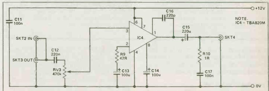
Fig. 4. The audio amplifier circuit. This section will prove useful for tracing signals, or testing small audio generator circuits.
