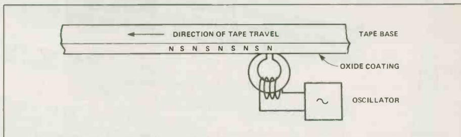
Fig. 1. The basic principle of tape recording.
