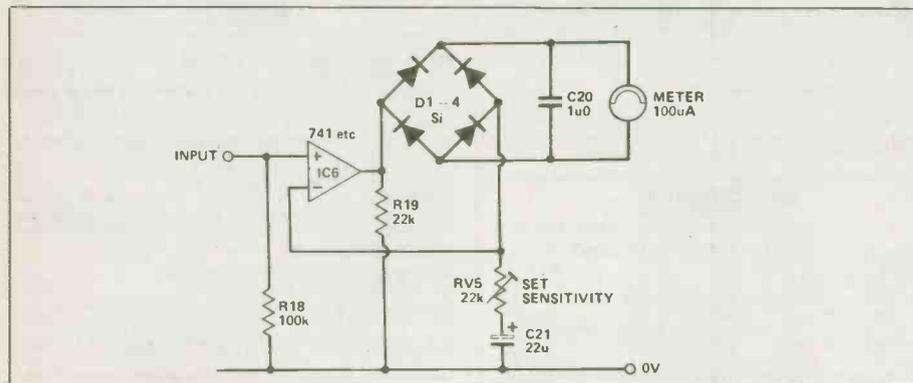
Fig. 16. A simple recording level meter circuit.
