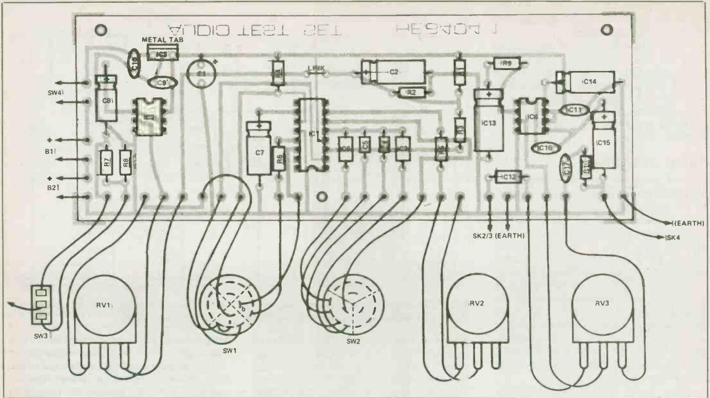
Fig. 5. All components, with the exception of panel mounted controls, fit onto a single small printed circuit board. Details of the connections from the PCB to the controls are also shown in the photographs below, and on the preceding page.
