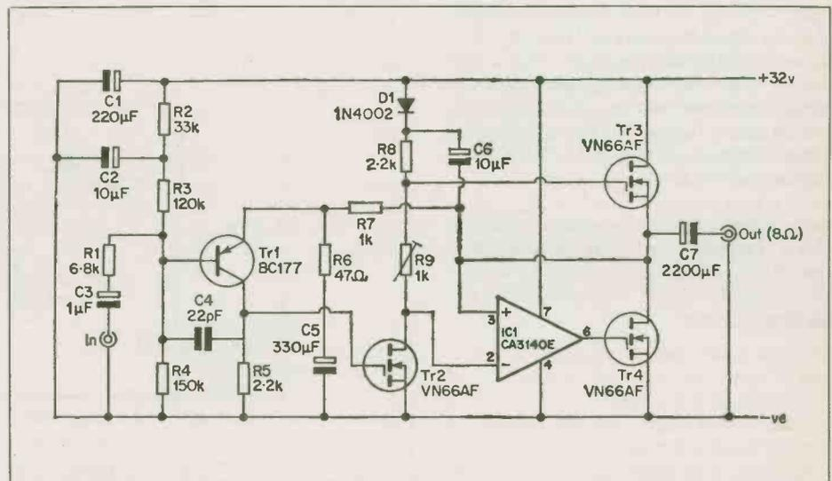
Fig. 4. A quasi-complementary VMOS amplifier giving 7 watts RMS.
