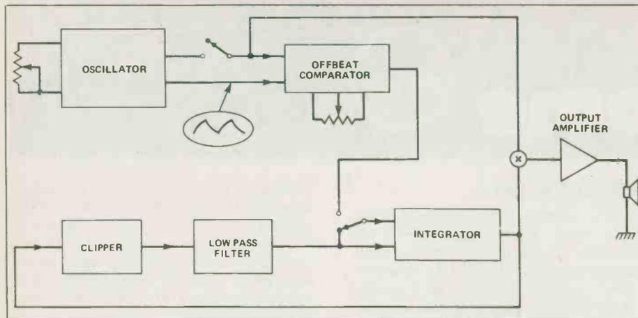
Fig. 1. The block diagram of the Offbeat Metronome.
