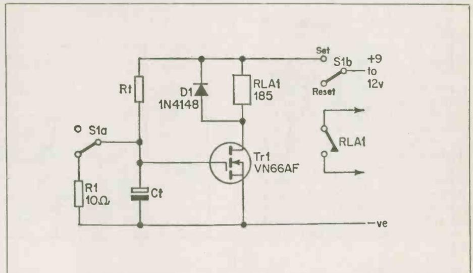
Fig. 7. An ultra-simple VMOS timer circuit.
