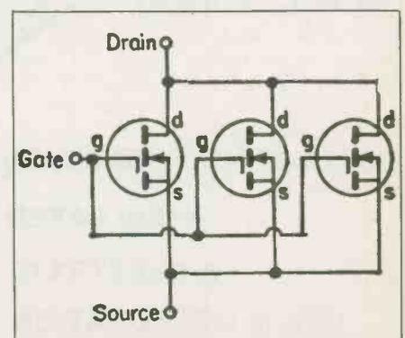
Fig. 2. VMOS devices can be added in parallel to reduce "on" resistance.
