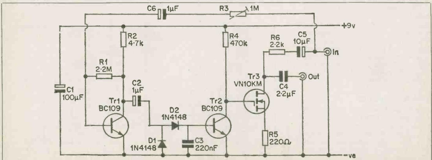
Fig. 8. The circuit diagram of the noise gate.
