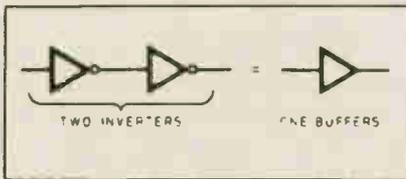
Fig. 13. Inverters connected in tandem.
