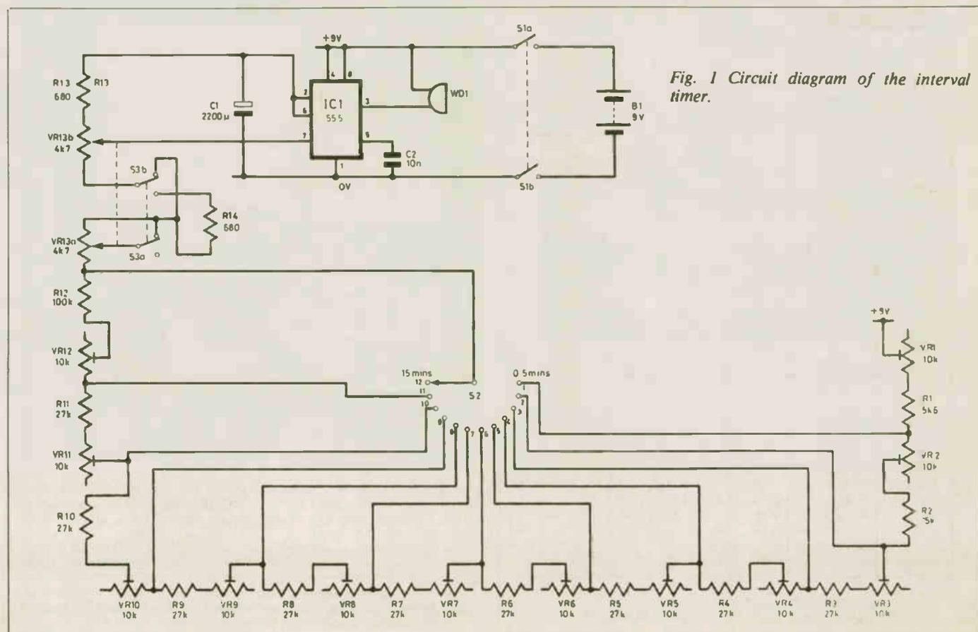
Fig. 1 Circuit diagram of the interval timer.
