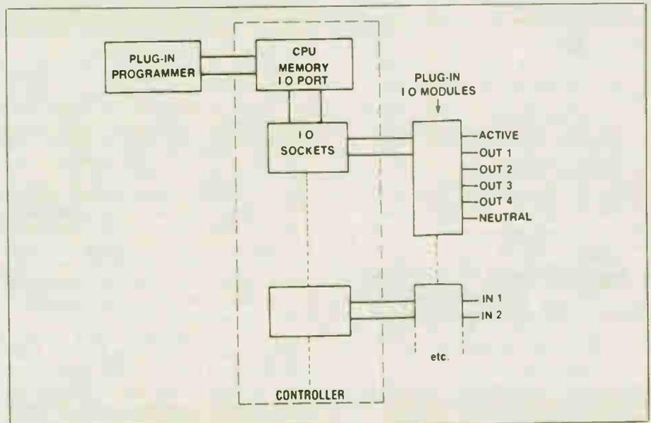
Fig. 3b. A typical P.C. used in practice.
