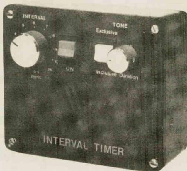
THERE ARE NUMEROUS occasions when it's useful to have some sort of timer which emits a signal at regular intervals. The circuit described here has been designed to fulfil this function in a versatile way, by providing a range of switched time intervals between 30 seconds and 15 minutes. The duration of the output tone can be varied so that a range of signals between a short burst and long tone can be obtained.
