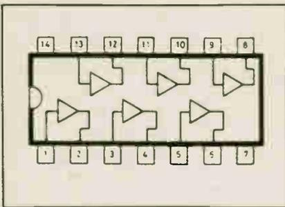
Fig. 10. Pin connector for a 7407 'hex' buffer.
