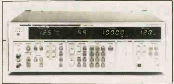
The LSG 245 AM Stereo Signal Generator from Leader Instruments provides a wide variety of modulation and output conditions, and is an ideal source for sensitivity, separation, selectivity, distortion and other tests on Motorola C-QUAM-type AM Stereo systems.
