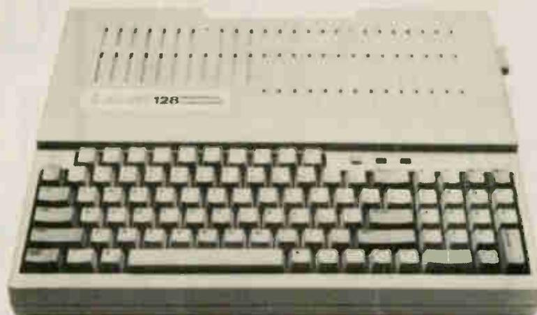
THE LASER 128 consists of the functional equivalent of an Apple IIe inside a case that's obviously been designed by taking a IIc package and adding a numeric keypad. The single included disk drive is a slot on the right hand side. The power supply lives in a small external box; it has adequate output to power the computer plus options such as another added drive.
