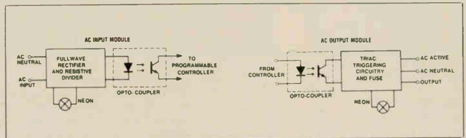
Fig. 5a. Block diagrams of typical I/O modules.
