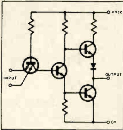
Fig. 5. Internal circuitry of a basic TTL gate.
