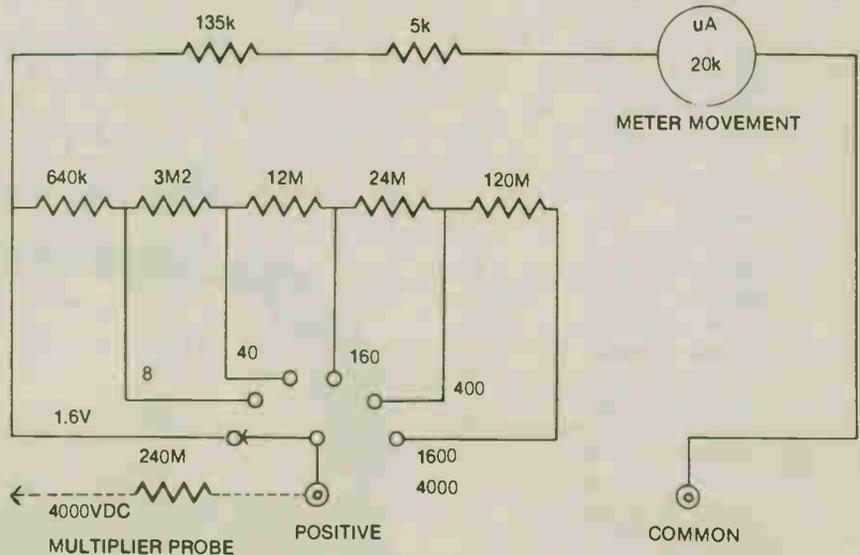
Fig. 1. A simplified DC voltmeter circuit.
