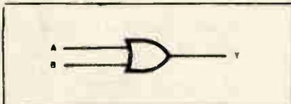
Fig. 21. Symbol for a two-input OR gate.
