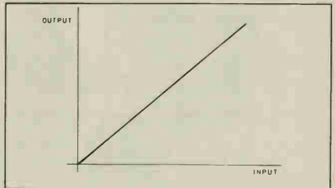
Fig. 4. Transfer characteristic for a conventional linear device.
