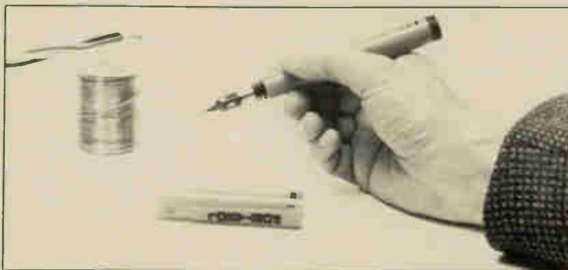
The incredibly talented hands in the photograph belong to the editor, who has just soldered three 16-gauge wires together using the Portasol Portable Soldering Iron. It's completely cordless, being powered by butane gas, the same stuff you use for lighters. In the cap (foreground) is a flint wheel lighter which ignites the gas after you thumb the on-off valve forward; the flame goes out in seconds, leaving a catalytic element to heat the tip flamelessly.
