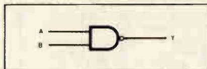
Fig. 25. Symbol for a two-input NAND gate.
