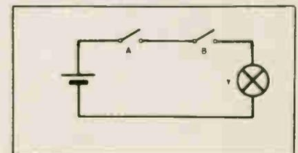
Fig. 18. Switch equivalent for a two-input AND gate.
