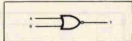
Fig. 28. Symbol for a two-input NOR gate.
