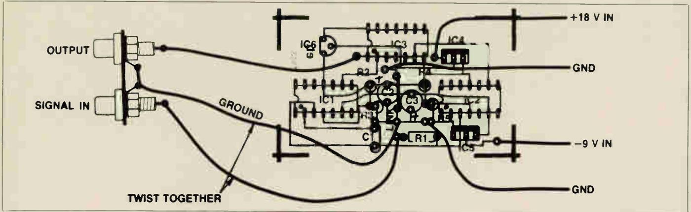
Fig. 3 The parts overlay for the frequency doubler.
