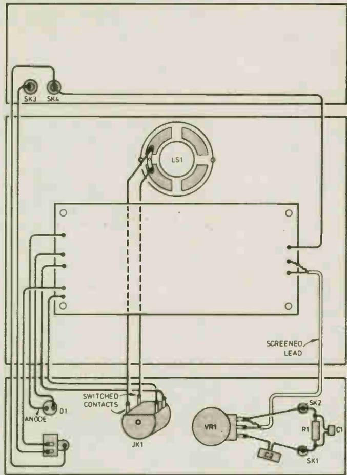
Fig. 4 Overall wiring diagram of the tracer.
