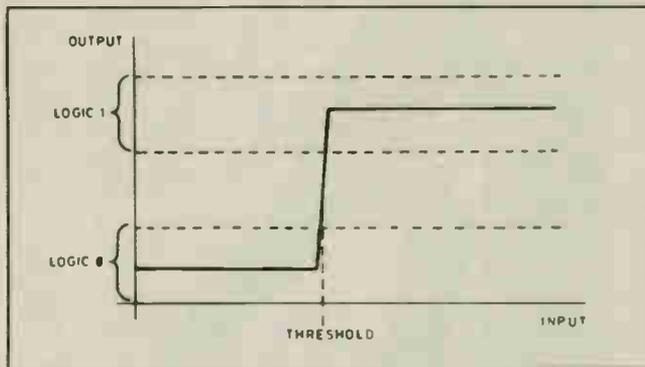
Fig. 3. Transfer characteristic for a typical logic device.
