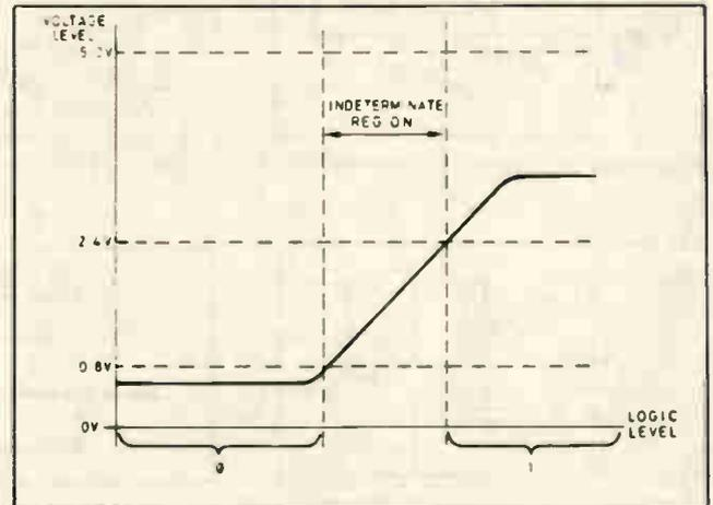
Fig. 7. Voltage characteristic for a TTL gate.
