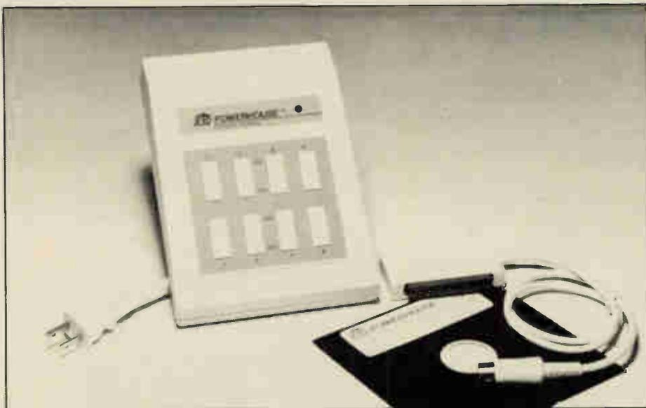
Fig. 1. The Powerhouse computer interface controls up to 256 appliance modules with a signal sent over the power wires.
