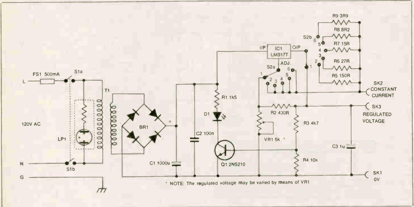
Fig. 3 Complete circuit diagram for the unit.
