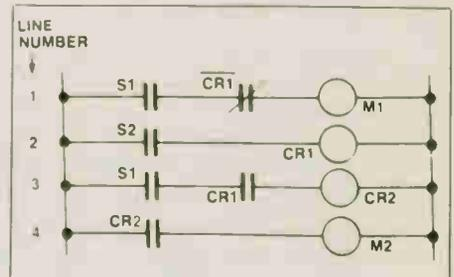
Fig. 2b. Relay ladder diagram for Figure 2a.
