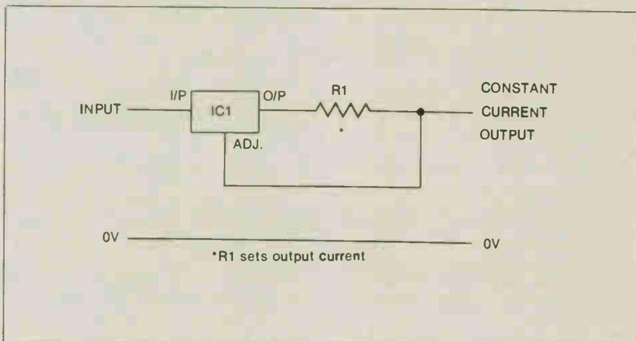
Fig. 2 Constant current regulation is determined by R1.
