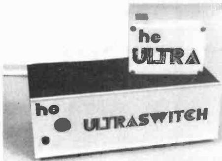
This project uses a 40kHz ultrasonic frequency to switch a relay at distances up to 20 feet. Modern circuitry keeps the component count low. The relay can of course control any equipment including a 110V socket.
