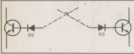
Fig. 3 Using base-isolating diodes to prevent base-emitter breakdown.
