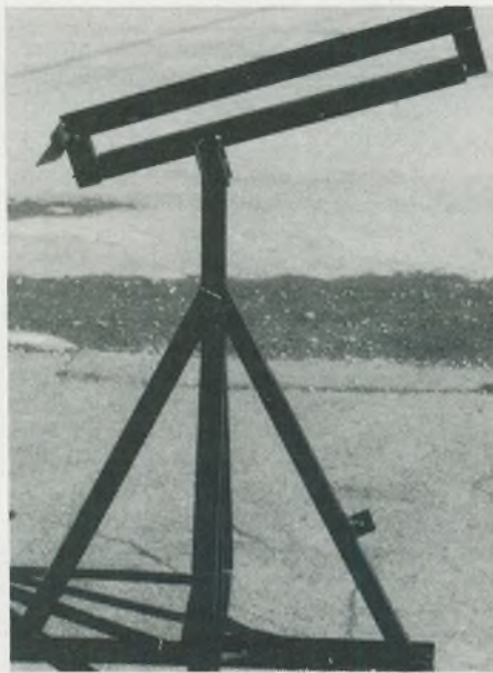
Fig. 5 The angle iron mount from Sothis Satellite plans.
