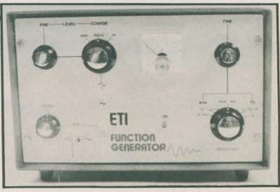
minals, each with its own attenuator network. A sine or triangle waveform is available from one output and a square wave is available from the other. The square wave output is available at all times, is synchronous with the sine/triangle waveform and can thus be used to provide synchronisation signals to an oscilloscope timebase during sine wave testing, etc. The unit is battery powered, for maximum user convenience.
