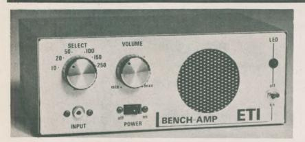
THE AMPLIFIER TO BE described here differs in one major respect to most others - it can be used as an accurate millivoltmeter! One of the most awkward things to measure in a lab is an audio signal of less than a volt. Specialist meters are expensive, and rarely justifiable for an amateur: hence this project. This provides at least an 'order of magnitude' reading, and in most cases an accurate value can be assigned to the signal.
