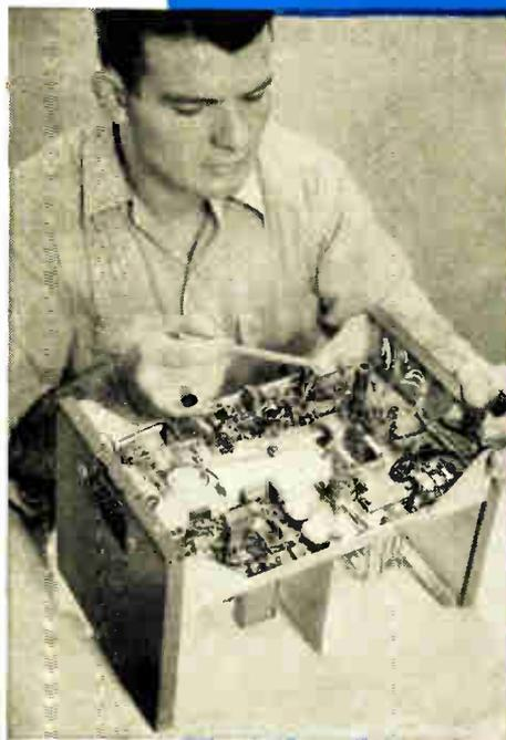
The underside of the Transmitter shows the freedom for inspection and maintenance. No component need be moved or removed to reach another.
