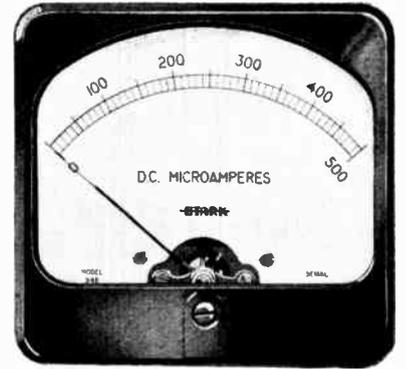
**MODEL 804.** DC volts, amperes, milli-amperes, microamperes. Moulded bakelite 4" rectangular case, flush mounting, spade or lance type pointer. Scale length 3.7" Also available in 3" rectangular case — Model 604. **NOTE:** High overload R.F. Meters also available with internal thermocouple.
