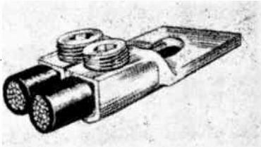
MU is produced from heavy, extra hard drawn seamless copper tubing by the IlSCO process. The copper is of 100 per cent electrical conductivity assuring low heat rise. MU has been tested by Underwriters Laboratories and the Canadian Standards Association.
