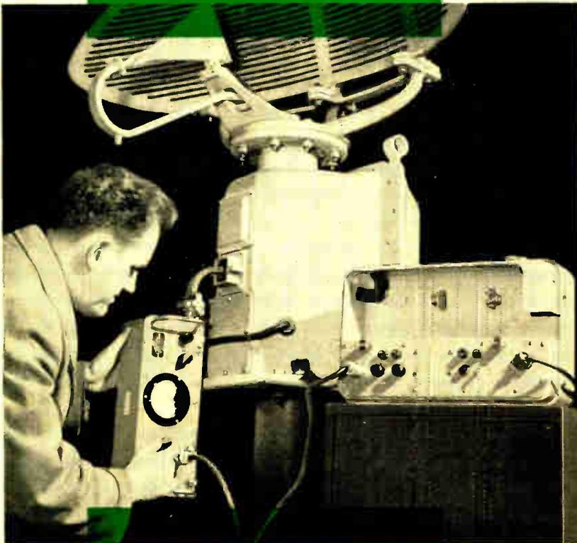
■ Now available is the Sperry Microline\* Model 539, VSWR Field Test Set, designed for accurate measurement of the voltage standing-wave ratio of X-band radar equipment during installation, maintenance and repair. This compact portable test set is also ideal for use in production and laboratory testing.
