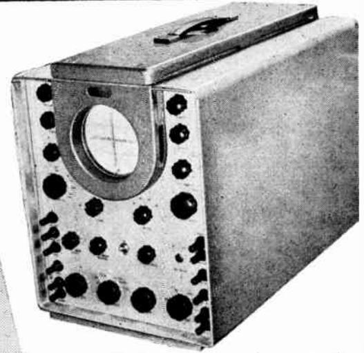
The Cossor Model 7514C oscilloscope is a versatile high gain wide band instrument for general laboratory and industrial applications. The model 7514C brings to this price range the accurate quantitative measurement found heretofore only in more elaborate and expensive equipment.
