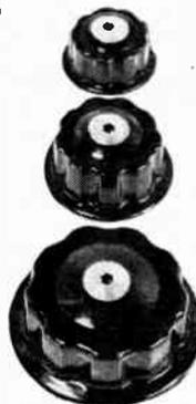
**1** **Bercostats.** A new range of power rheostats for industrial electronics. 5 sizes from 25 to 150 watts. All ceramic construction. Windings embedded in vitreous enamel giving great mechanical strength. Finishes comply with RCS.1000. Available in open, protected and ganged models.
