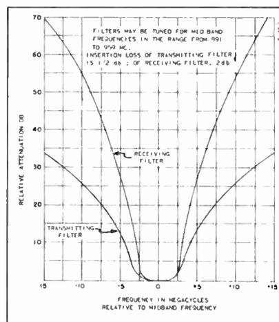
● Figure 2. The transmitting filter consists of two tuned cavities in series. The receiving filter consists of four cavities in series.
