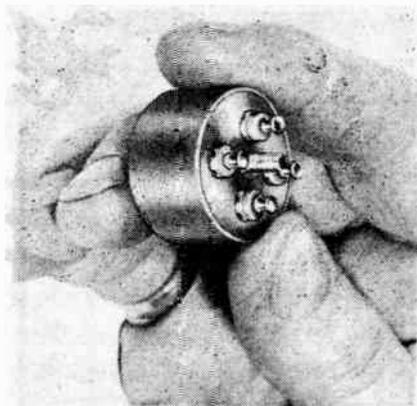
weighs but 1 1/2 oz. Electrical ratings are: Input, 115 volts, 400 cycles; Power output, 6 VA; Regulation, 10 per cent; Heat rise 40°C. Class "A". It is hermetically sealed in a metal case to MIL-T-27 requirements.
