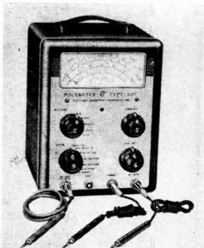
The flexibility of this instrument is increased by its ability to read peak to peak voltages directly. The accurate measurement of the peak to peak value of many complex waveforms makes the 301 indispensable to the TV service man in trouble-shooting Video, Sync and Deflection circuits.
