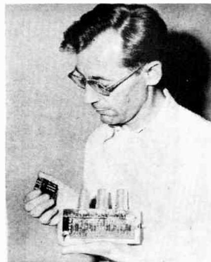
● Comparison of transistor and conventional tube circuit.
