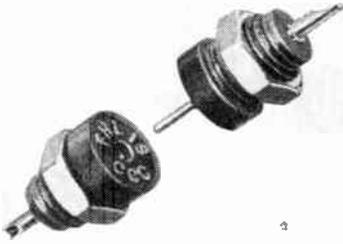
The extremely rugged "FHL" has high dielectric characteristics and features the use of one-piece moldings available in three insulating materials: Mineral (asbestos) filled Melamine for high dielectric and mechanical strength, Plaskon Reinforced (glass) Aklyd type 440A for unusually high impact strength and arc resistance, and Diallyl Phthalate (blue) with high dimensional stability plus excellent dielectric properties.
