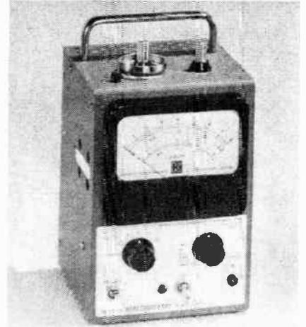
All Keithley Electrometer accessories fit the new model. It can thus be used not only as a dc voltmeter, but as an extremely sensitive micromicroammeter, megohmmeter, and Kilovoltmeter. Maximum full-scale sensitivities are  $8 \times 10^{-13}$  ampere,  $3 \times 10^{11}$  ohms, and 20,000 volts.
