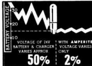
Amperite Regulators are the simplest, most effective method for obtaining *automatic regulation* of current or voltage. *Hermetically sealed*, they are not affected by changes in altitude, ambient temperature ( $-55^{\circ}$  to  $+90^{\circ}$  C), or humidity. Rugged; no moving parts; changed as easily as a radio tube.
