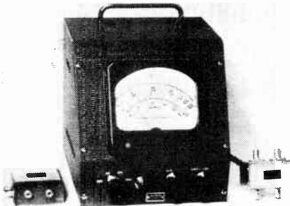
light weight and convenience of operation. In particular, it will be invaluable in measurement of: Vector sum or difference of two voltages; phase angle between two voltages; voltage between two points which are both at a.c. ground potential; magnitude and phase angle of an unknown impedance. Accuracy:  $\pm 5$  per cent nominal; error increases as frequency is approaching 1000 Mc/s.
