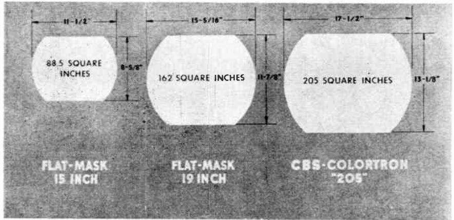
● Flat-mask color tubes and the "205" are compared to show the large increase in useful picture area attained by CBS-Hytron's original curved-mask design.
