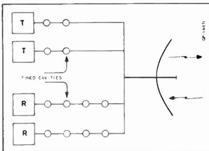
● Figure 1. Block diagram of two transmitters and two receivers diplexed over a common antenna by the use of tuned cavity directional filters.
