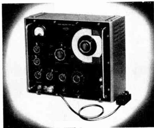
This instrument is a selective measuring set of great versatility operating over the frequency range 30 kc/s - 30Mc/s. It consists essentially of a stable high-gain selective amplifier, operating on the heterodyne principle and incorporating H.F. and L.F. attenuators. The output in the form of an audio frequency is applied to a meter circuit and to headphones.
