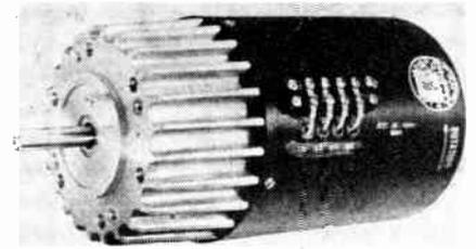
430 inch ounces at 1475 RPM. Locked rotor torque is 500 inch ounces at zero RPM and pull-out torque is 700 inch ounces at zero RPM. Motor is fan cooled on a totally enclosed frame, shaft and hardware is of stainless steel and ball bearings are employed throughout. Weight is 22 lbs.
