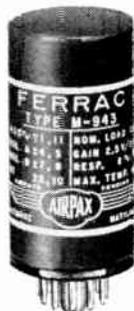
**MAGNETIC AMPLIFIERS** for instrumentation and control are unusually stable. Design of mixing, lead, and lag networks to work with these amplifiers is straight-forward. Normal gain of Type M-943 is 2.5 volts  $\pm$  1 db of output for each 100 microamperes of input. Units draw less than 3 watts from 400 CPS supply, occupy about 6 cu. in.
