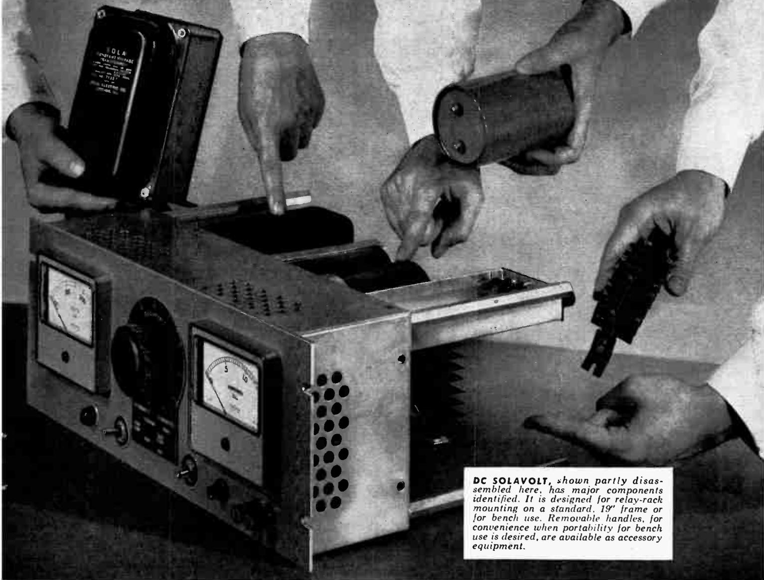
**DC SOLAVOLT**, shown partly disassembled here, has major components identified. It is designed for relay-rack mounting on a standard, 19" frame or for bench use. Removable handles, for convenience when portability for bench use is desired, are available as accessory equipment.
