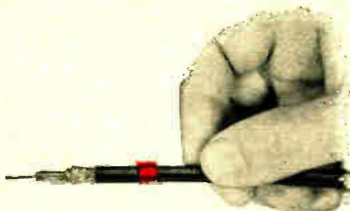
**INSERT** ground lead under outer Hyring and line up over the inner Hyring.
