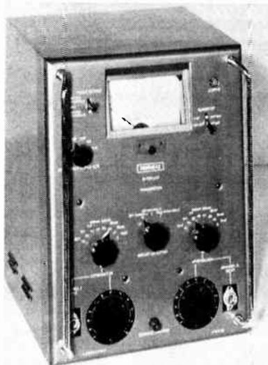
(1mV to 20V), Q-measurements using simple external equipment, expansion of the degree scale in the region of 0° and 180° and the measurement of the in-phase and quadrature components of an input signal. Relevant literature: Publication 9720. A low-frequency version (0.5c/s to 10kc/s) is also available.
