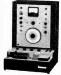
**MEGOHMMETER** range from 100K to 10,000,000 Megohms, test voltage 10 to 100 V. Can be used as D.C. Voltmeter from 10mV to 2000 V with 1000 Megohm input impedance. Illustrated with high tension accessory extending range to 100,000,000 Megohms and voltage from 0-1000.
