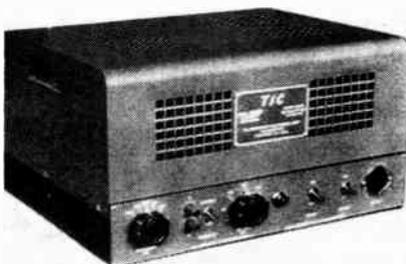
and from 200 to 1700 c.p.s. by means of an external capacitor. The frequency of the 250, 500 and 1000 v.a. units is continuously variable from 330 to 3700 c.p.s. in five ranges. Output amplitude is continuously variable from 90 to 130 volts.
