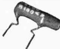
Available with crimped leads, for printed wiring board insertion
