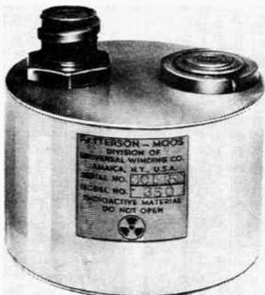
The heart of the Timer is a Nuclear Battery which has been in production at the Patterson Moos Division for the last few years. This battery converts nuclear energy directly into electrical energy. It is made with current ratings from 50 to 5000 micromicroamperes and equilibrium voltages in the order of 10,000 volts. Battery performance is not affected by environmental conditions, and shelf and use life are not changed by short circuiting.
