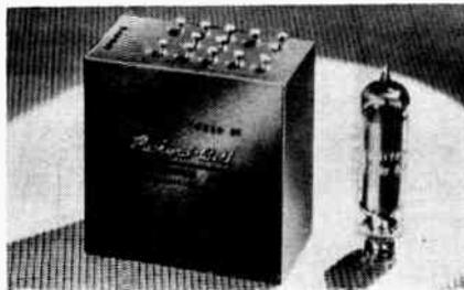
The custom component has a life expectancy of 10,000 hours or more, with ripple less than 50 mv from peak to peak, operating temperature of minus 65 degrees to plus 125 degrees centigrade, and is adaptable to voltages of plus or minus 50 to plus or minus 1000. Its regulation is plus or minus 1 per cent, with circuit gain of 60 to 80 db.
