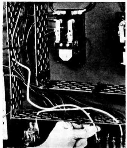
snapped on. Channel-Duct replaces hand-formed solid wire layouts, eliminates expensive harnesses and simplifies maintenance. It is easy to shear, easy to mount and doesn't require mitred corners.
