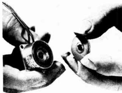
No slip rings or brushes are required for the SF-100 clutch since the flange-mounted field is connected through pigtail leads to a 28- or 90-volt d-c source. In the clutch, torque is transmitted through the rotor to the armature which may be keyed to the driving or driven member. Power required is 6 watts maximum.
