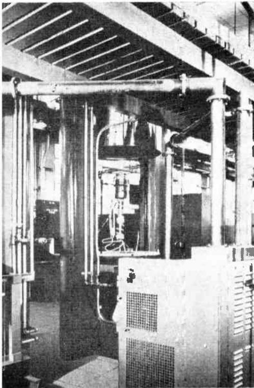
● An installation in which coaxial cable has been used to effectively solve many of the inherent electrical problems previously encountered in induction heating.
