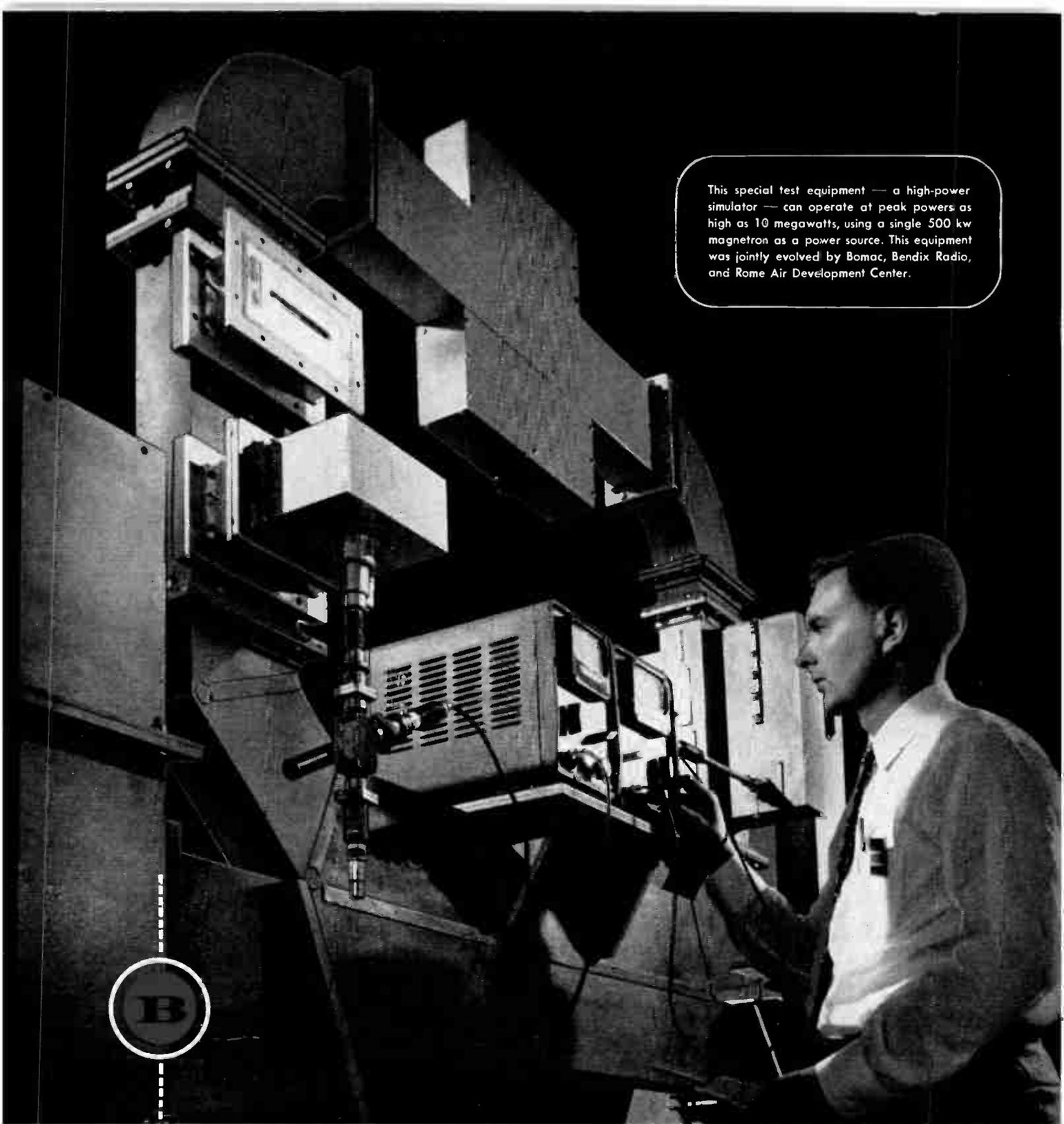
This special test equipment — a high-power simulator — can operate at peak powers as high as 10 megawatts, using a single 500 kw magnetron as a power source. This equipment was jointly evolved by Bomac, Bendix Radio, and Rome Air Development Center.
