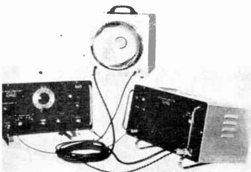
The equipment consists of a variable frequency oscillator and a high intensity stroboscope. The oscillator provides a sine wave output to drive a separate power amplifier and vibrator generator.
