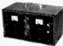
Will supply either 6 or 12 volt output to take care of auto radios on even the most modern cars. Output voltage is variable from zero to 8 volts DC or 0 to 16 volts DC. Will deliver up to 15 amperes at 6 volts or up to 7 amperes at 12 volts. Two 10,000 microfarad output filter capacitors insure smooth DC output. Panel meters monitor output current and voltage. Will double as a battery charger.
