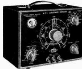
**BJ-1**—Checks all kinds of condensers for capacity, leakage, opens, shorts or intermittent conditions. Direct reading .00001 to 1000 MFD. Resistance from 100 ohms to 5 megohms. \$34.95
