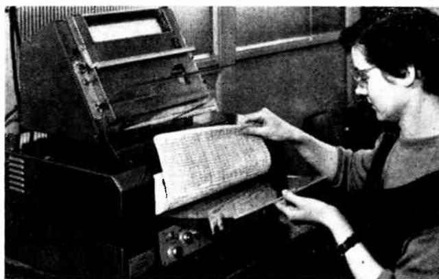
(Above) The transmitter drum being loaded with information to be transmitted. (Left) Transmitted information being received on the receiver unit of Mufax equipment. Photos courtesy — Rolls Royce Limited.
