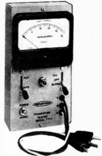
The unit provides an easy-to-read sensitive 50 microampere movement mounted in a sturdy case, is entirely self-contained, and requires no external power connection.
