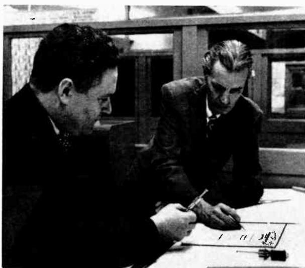
*(Above) Engineers check the mechanical tube dimensions against drawings.*
