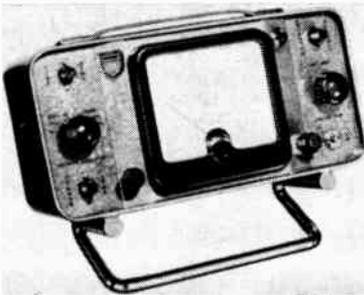
It is claimed by the manufacturer to be the only meter available which covers all DC voltages present in modern television and radar equipment.
