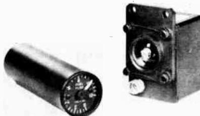
Developed for the U.S. Army through Wright Air Development Center under a U.S. Air Force contract by General Electric's Instrument Department, the small, lightweight system has only two basic components — a type TJ-64 flowmeter transmitter and a type DJ-99 remote indicator.
