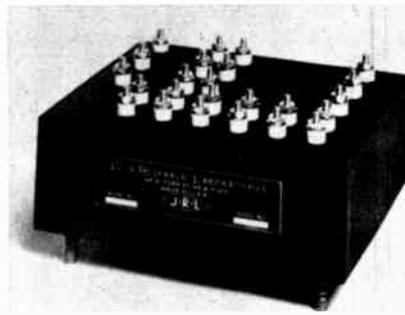
An oil-bath construction is used to minimize thermal and self-heating effects. The total effect of all transient thermal influences, including self-heating, Seebeck, and Peltier effects, is less than .0005% of full scale.
