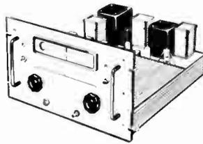
*45 Mc/s; Sensitivity: 25 MicroV. for a 12 db signal to noise ratio; R.F. Gain: 12 db; I.F. Gain: 80 db; Image Rejection: 40 db; Input Impedance: 75 ohms (approx.) Unbalanced; Output Impedance: 80 ohms (approx.); Outputs: (a) 0.5v from Crystal Detector, (b) 300 mV at 45 Mc/s.*
