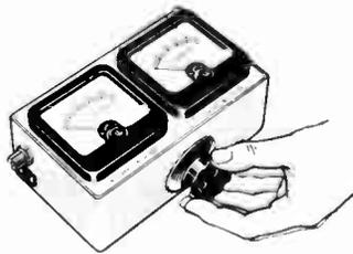
*Accuracy (at frequency of calibration): low range 0.1 db, high range 0.2 db; Directivity: 26 db (approx.); Coupling Coefficient: 30 db (approx.).*
