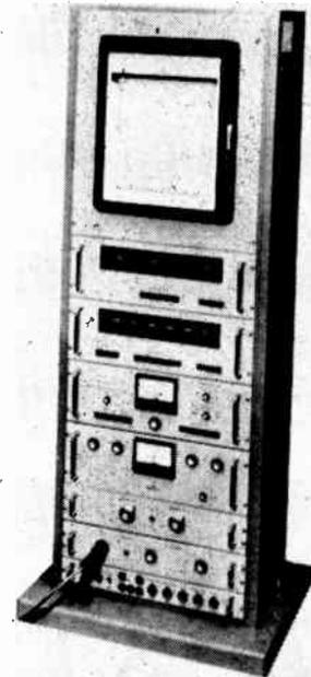
The P.H.A. provides an electronic means of discriminating against either low or high amplitude pulses, resulting in improved peak-to-background ratios with minimal loss of radiation intensity.
