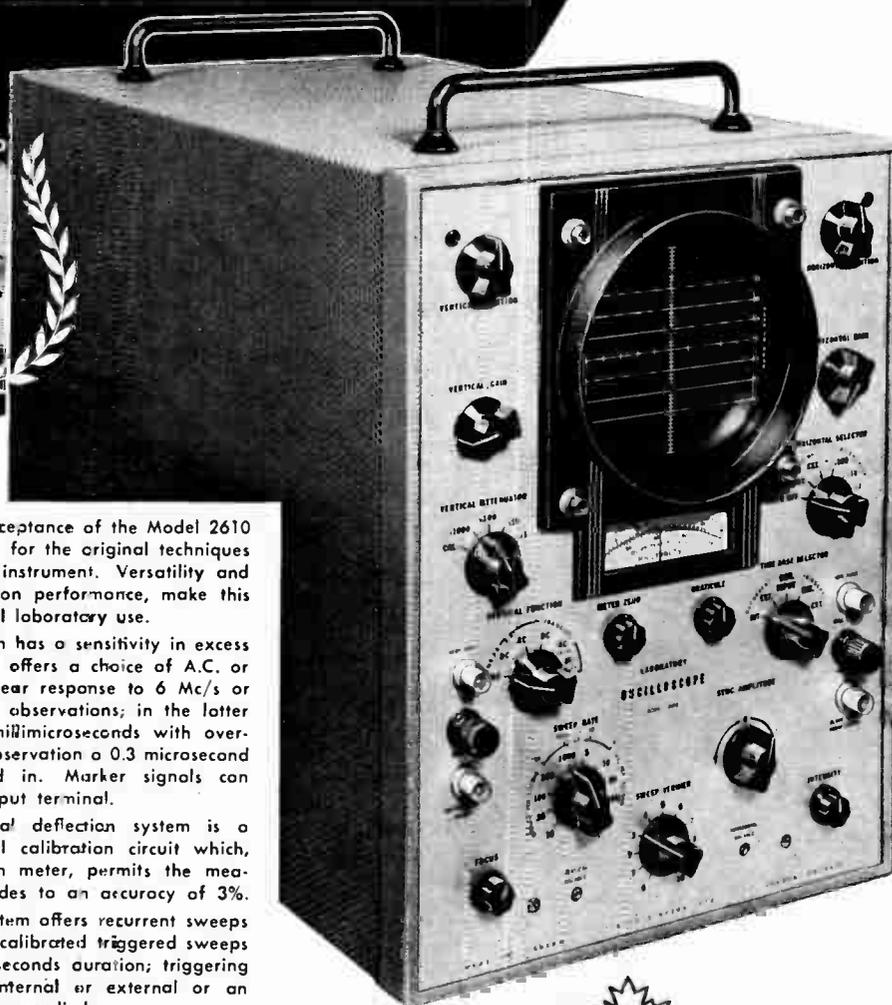
The wide and immediate acceptance of the Model 2610 has provided ample justification for the original techniques adopted in the design of this instrument. Versatility and convenience, allied with precision performance, make this an ideal oscilloscope for general laboratory use.
