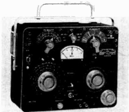
One important feature of the Type 1650-A is Orthonull, an exclusive new mechanical-ganging device which facilitates measurement of low-Q inductors (or high-D capacitors). Orthonull adds convenience and accuracy and makes easy many low-Q measurements that are practically impossible on other impedance bridges.
