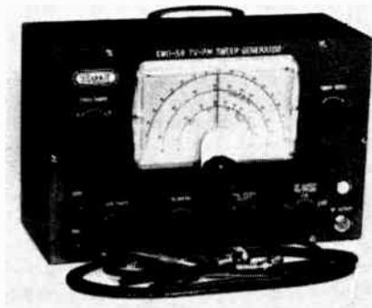
Sweep width is continuous from 0 to 12 MC on all frequencies and incorporates phasing and blanking control. When combined with its twin, the STARKIT Model MHG-48 Marker Generator, and an oscilloscope, accurate response curves may be obtained.
