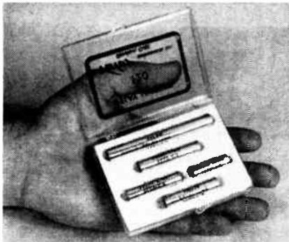
consists of five lumped constant delay lines of 0.1, 0.2, 0.3, 0.4, and 0.6 US delays with .05, .06, .07, .08, and .09 US rise times respectively. The delay lines may be used individually or they may be series connected to give any delay from 0.1 microseconds to 1.6 microseconds. For further details write: A. Deskin Sales Company, 6875 Fielding Avenue, Montreal, Quebec, Canadian Sales Representatives.
