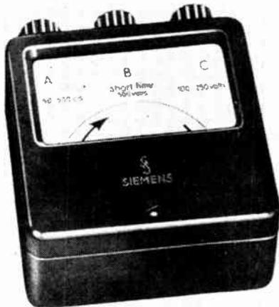
above the magnet poles. When the instrument is connected to three-phase current, the magnet poles generate a rotating field driving the disc. The rotation of the latter can be observed through the window of the instrument.
