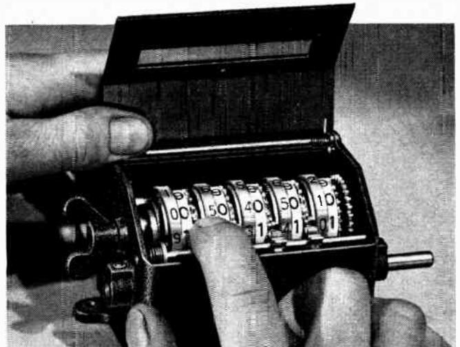
The High Speed Predetermining Counter is the basic counter in this complete line. It provides automatic control by this simplified method: . . . to set a run of 5451 pieces on the counter: (1) Set all white wheels to zero with one turn of wing-nut; (2) Now, set the metal wheels, one by one. Set first wheel to "5", opposite zero on its "opposite number" white wheel, then set the "4", "5" and "1" and that's all . . . you're ready to throw the switch and start the run.
