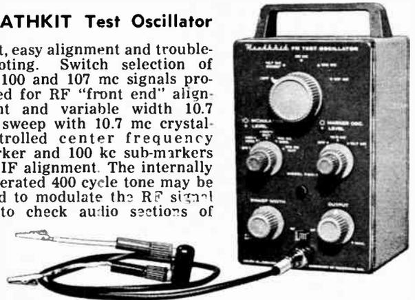
receiver. The 10 mc crystal-controlled oscillator signal is used to calibrate the instrument and is also available separately for use as a standard in calibrating other equipment. 400 cycle AM modulated 10.7 mc signal allows easy alignment of ratio detector and discriminator transformers. 5 lbs.
