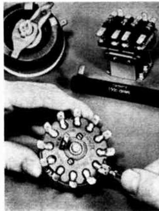
Such connectors (also known as quick-disconnect terminals) are produced by a number of electrical hardware manufacturers. Automatic machinery is available to fasten these connectors to the leads at high speed thereby offering important time savings.
