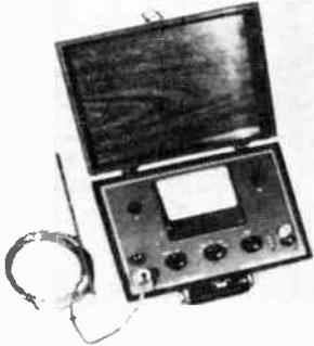
Model 54A1 measures average and instantaneous velocities in the flow of air by making use of the cooling effect of the stream on a thin electrically heated wire filament. A completely transistorized circuit maintains constant the resistance ratio of a hot and cold filament.
