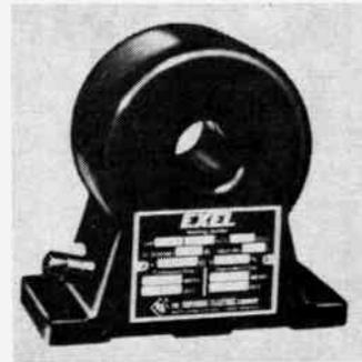
Essentially, an Exel consists of a gapped, strip-wound silicon steel toroid core, wire-wound and imbedded in epoxy compound. The entire assembly is enclosed in a compact phenolic case having two Superior 5-way binding posts for connections. Dimensions are 6" L x 2 5/8" W x 5 3/4" H.
