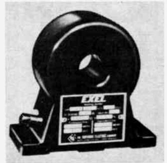
Essentially, an Exel consists of a gapped, strip-wound silicon steel toroid core, wire-wound and imbedded in epoxy compound. The entire assembly is enclosed in a compact phenolic case having two Superior 5-way binding posts for connections. Dimensions are 6" L x 2½" W x 5¾" H.
