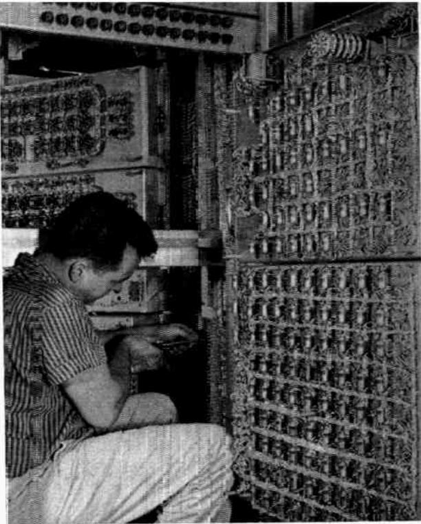
Fig. 5. The complexity of the electronic equipment which makes up the BMEWS surveillance radar sub-system is evidenced by this RF Switching cabinet shown being assembled at the General Electric Company's plant.
