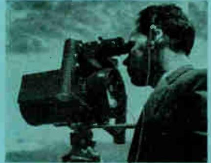
and research roles to determine temperature differences or (in modified form) to make accurate temperature measurements. One version has been used as an intrusion alarm. The instrument normally may be mounted on a tripod while it is being used.
