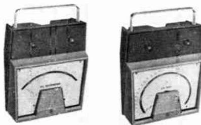
corporation of taut-band suspension mechanisms eliminates pivots and jewels, the most expensive instrument maintenance factor. Repeatability of readings is better than 0.05 per cent since friction is entirely eliminated.
