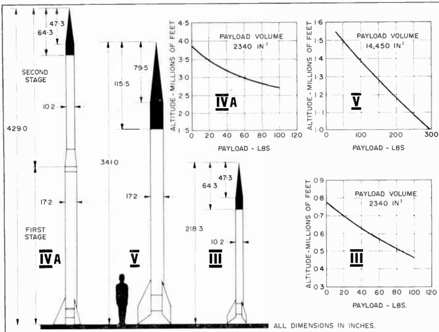
Figure 2. Three members of the Black-Brant family of rockets showing payload/altitude performance. Black area at the rocket nose shows the payload compartment.
