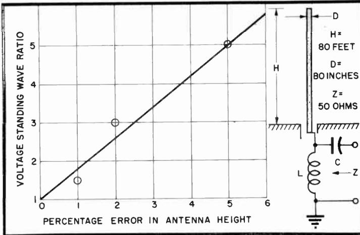
Figure 7. Relationship between mast height mismatch and VSWR for the tubular antenna.
