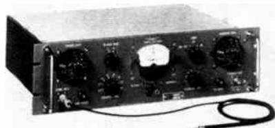
ture voltage ratios of any 3- or 4-terminal network. Accuracy of in-phase measurements is greater than .01 per cent of range. Quadrature accuracy is greater than .1 per cent of range (plus calibration error and .0002 Rx).
