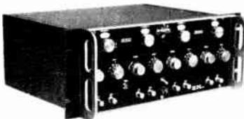
Abtronics Model 100 is a general purpose laboratory delay unit designed for use with the Model 2 camera to trigger delayed shutters or fire such auxiliary equipment as flash guns. It is also useful in camera systems where a number of photos are being taken at remote points and/or in sequence. Combining the delay unit with the new low price Model 2 camera offers the user exceptional flexibility and economy in the design and construction of camera systems.
