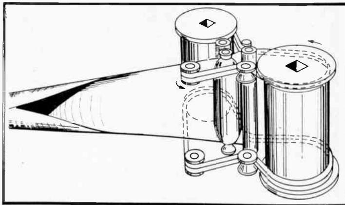
Figure 2. Diagram showing principle of tube extension for designs employing spring or rubber belts.
