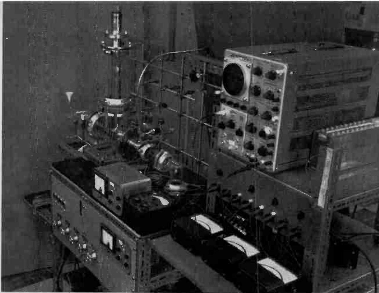
Figure 1. Experimental set-up for producing  $SF_6$  negative ions for charge neutralized ion engine.
