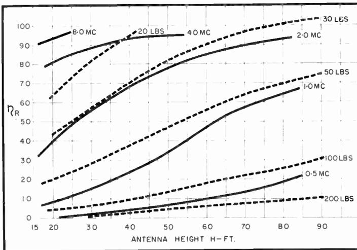
Figure 8. (above) Efficiency against antenna height for antenna lengths less than  $\lambda/4$ . Chart also shows weight of inductive matching unit.
