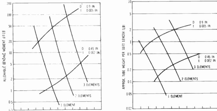
Figure 6. (left) Allowable bending moment as a function of tube dia. and (right) tube dia. versus weight.
