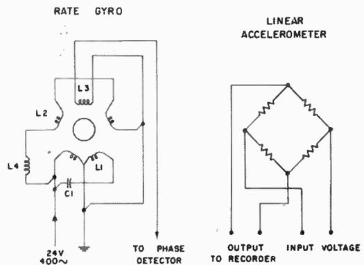
Figure 2. (above) Diagram of helmet gyro and linear accelerometer. Figure 3. (below) Circuit diagram of the phase sensitive detector.
