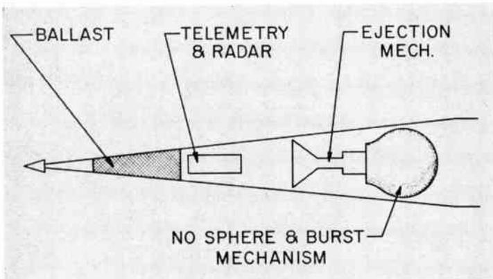
Figure 6. Layout of Nitric Oxide (NO) seeding nose-cone.
