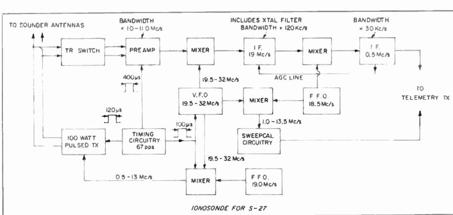
Figure 2. (left) Block diagram of the ionosonde system of the S-27 satellite. Figure 3. (lower left) Diagram showing the satellite's telemetering system.
