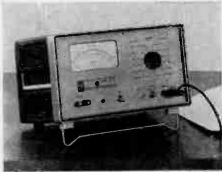
Sierra Electronic Corporation, division of Philco Corporation, Model 127A Solid State Selective Voltmeter. Covers 2-350 Kc/s, -80 to +22 DBM, accuracy  $\pm 1$  db, built-in crystal calibrator, rechargeable battery, light and portable.
