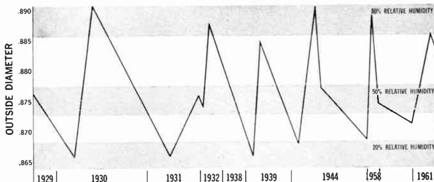
Long term test of fibre, which has been going on since 1929, shows that fibre still responds to wide humidity changes in the same way it did when test began. Predictable changes in dimension occur when fibre tubing is subjected to extremes of humidity. Tests such as these prove that there is no change in Vulcanized Fibre characteristics over long periods of time.
