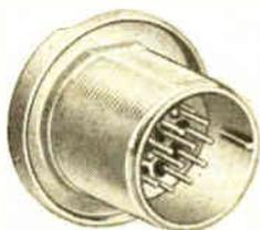
**HERMETICALLY SEALED** Available in most popular plug lines. Includes the first Series approved to MIL-C-25955, which requires leakage rates of less than .001 micron cubic foot per hour ( $1.5 \times 10^{-8}$  cc/sec.). Plugs for all hermetic applications—standard or custom designs, with some series designed to withstand extreme thermal shocks, temperatures from  $-100^{\circ}\text{F}$  to  $1000^{\circ}\text{F}$ , pressures above 2000 psi.
