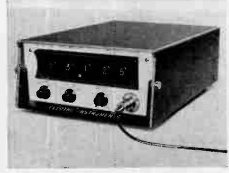
Sierra Electronic Corporation, Div. of Philco Corporation, Model 126A Frequency Selective Voltmeter 5 to 1620 Kc/s, -90 to +32 DBM dual selectivity, carrier reinsertion and crystal calibrator built-in.
