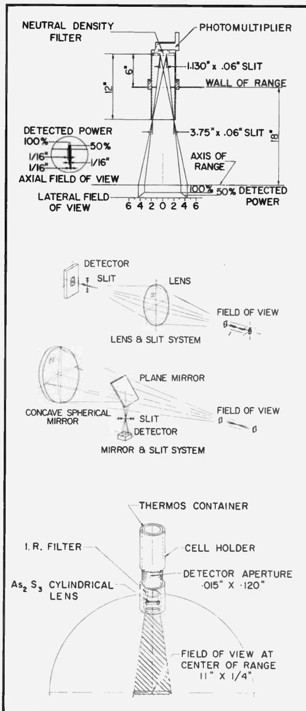
of an inch. Nevertheless, this simple, sturdy and inexpensive construction has many qualities which render it attractive for stagnation point radiation studies and as a trigger initiator. These qualities consist of high transmission which is practically independent of wavelength, a high aspect ratio field of view and an infinite depth of field, which is especially advantageous when used as a trigger generator.
