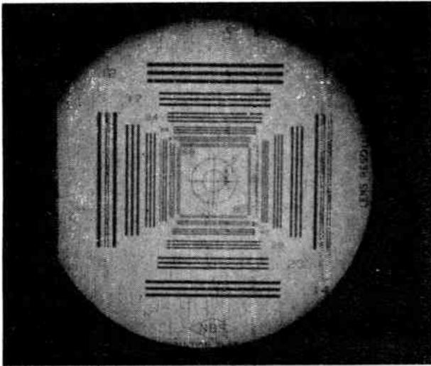
This is an actual size portrait of an NBS resolution chart taken at 0.1 microsecond with an Abtronics electronics framing camera
