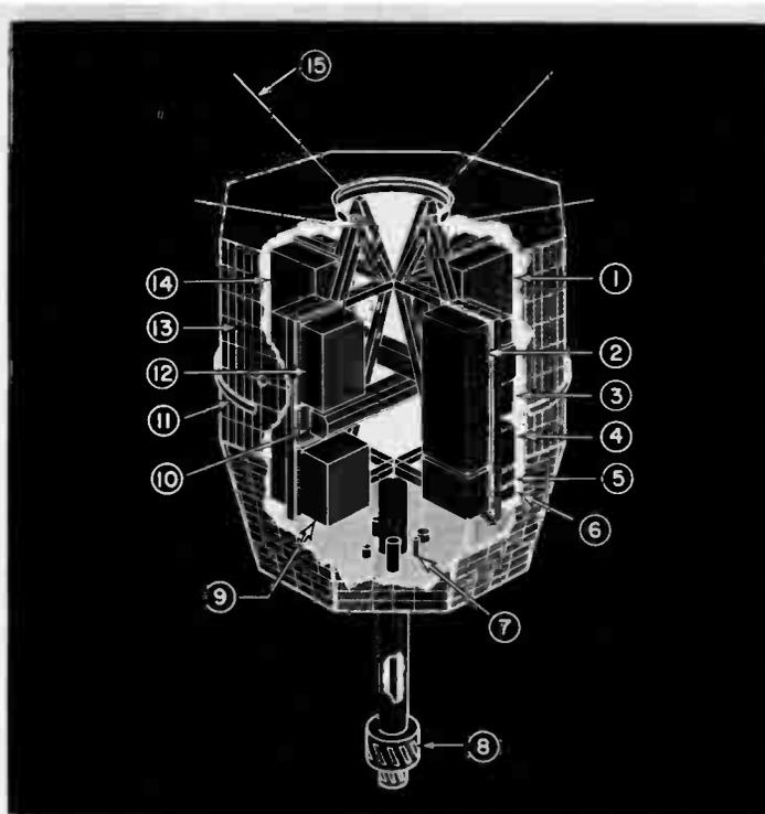
Figure 2. Diagram showing main components of the RELAY I satellite:
