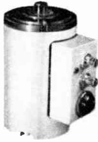
Norden's new MICROGON provides digital encoding of angular displacement and angular rate with continuously available pure binary or binary-coded decimal output in parallel or serial form. A new electronic technique for coarse angle data acquisition allows all angular information to be carried over only two wires from the transducer. Standard resolutions are 360,000 counts per turn  $2^{19}$  cpt.
