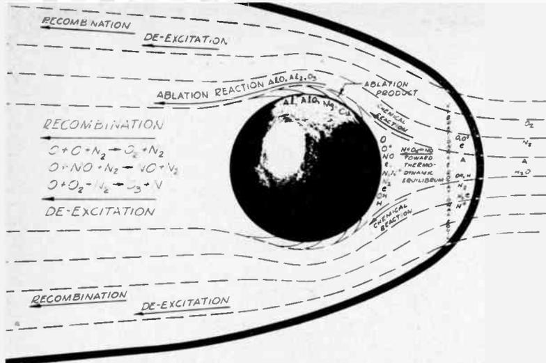
Figure 2. Diagram showing the various processes occurring in the luminous volume surrounding hypersonic bodies.
