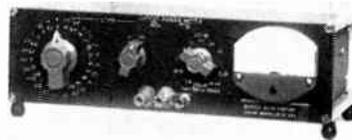
cade power ranges are available from 0.1 mw to 20 w. An auxiliary scale reads from -10 to 43 db re 1 mw. This meter has a quasi-rms response.
