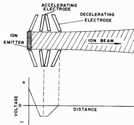
Figure 3b. The "accel-decel" ion-engine structure and diagram showing voltage distribution.
