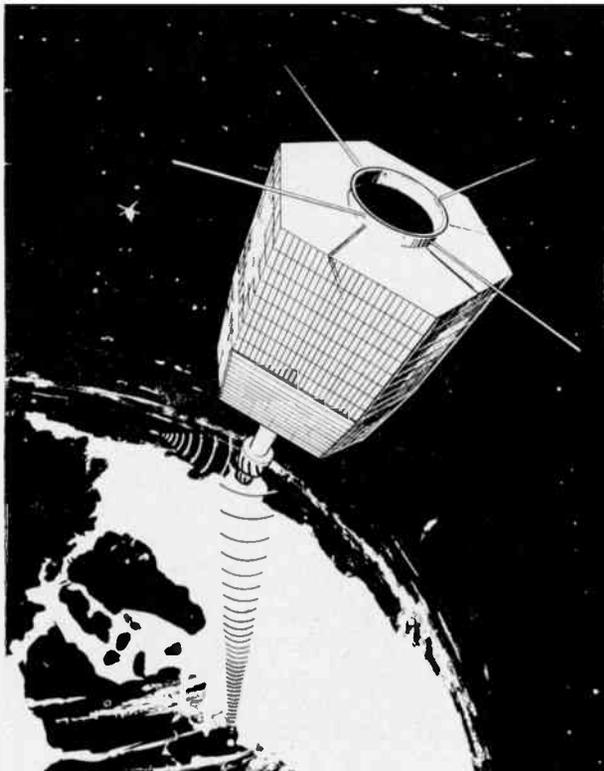
Figure 1. Impression of the RELAY satellite in orbit passing over the Atlantic and linking Europe with North America by line of sight communication.
