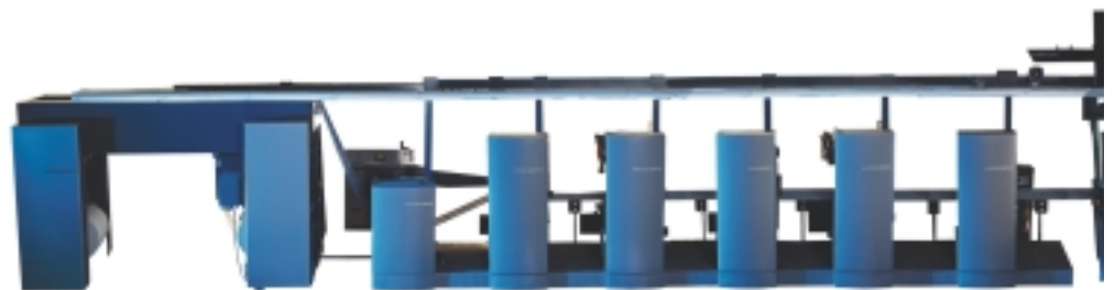
Heidelberg M-130 5-colour heat-set web press
