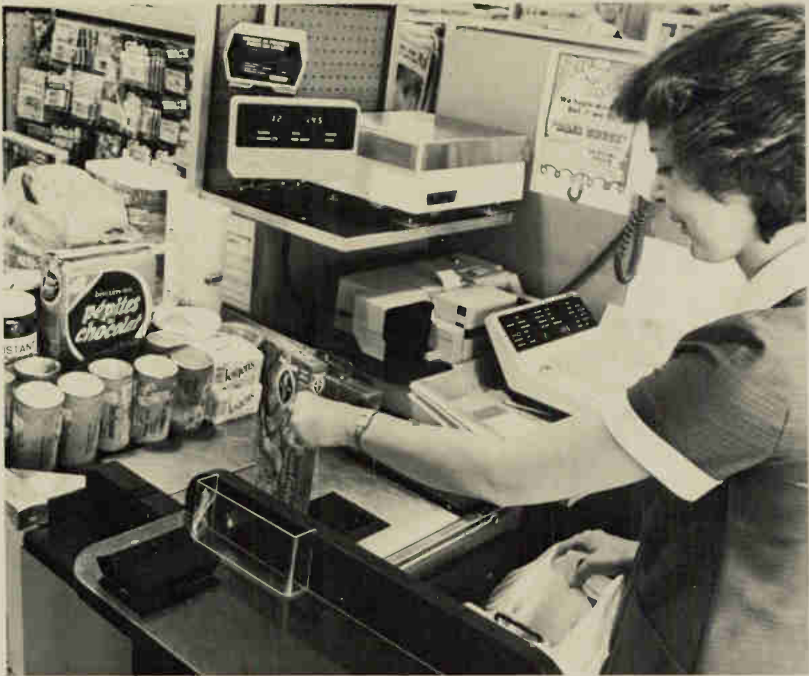
Scanning devices and front-end checkout units are the most visible part of the move to wider use of POS equipment. Shown is an installation at Food City store in Oakville, Ont.
