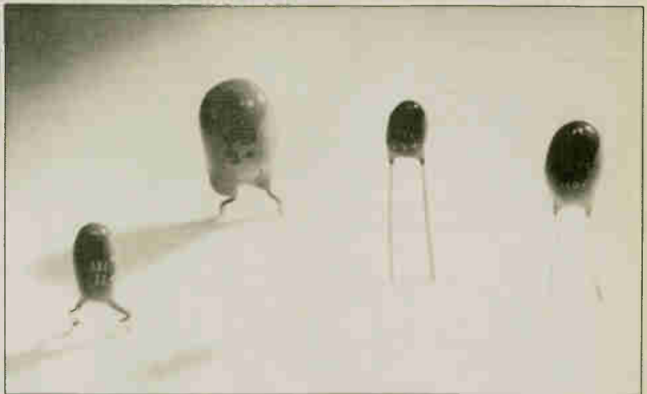
Fig. 5 Various tantalum bead capacitors. The long lead indicates the positive connection.
