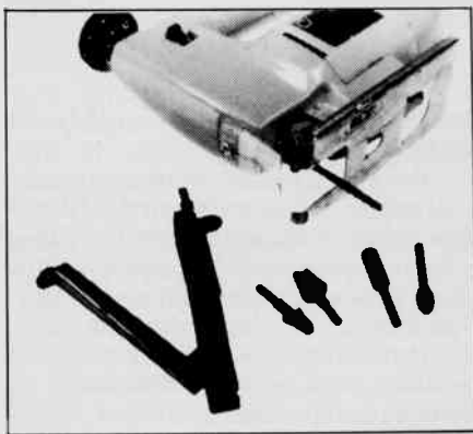
Some metal-working tools to make life easier: the Adel nibbler, a sabre saw, two conical cutters and two rasps that fit power drills.
