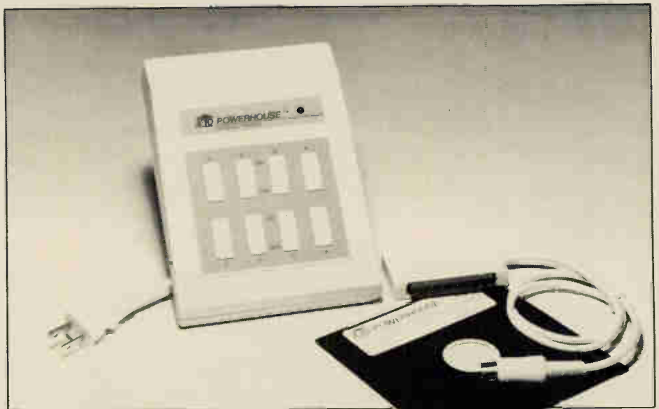
Fig. 1. The Powerhouse computer interface controls up to 256 appliance modules with a signal sent over the power wires.
