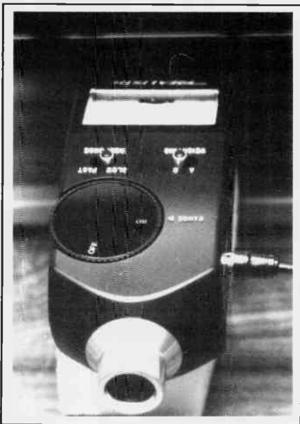
The output of the meter is fed into a scope; at the moment it's reading the whirring of the camera shutter.
