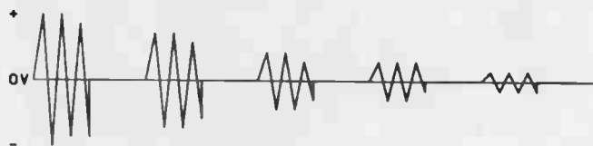
Fig. 1. (above). A combination of the signal's natural decay and the chopping effect of the unit gives an echo effect.
