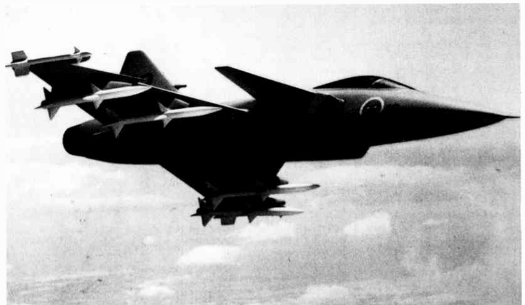
The model shows the JAS-39, Sweden's sixth generation of Swedish-developed fighters. It employs large areas of graphic composition in its airframe.
