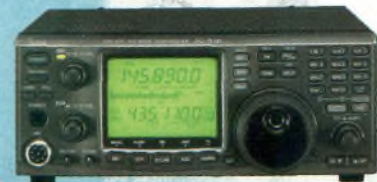
IC-910H VHF/UHF tous modes 100 W (VHF) et 75 W (UHF) Option 1200 MHz (10 W)
