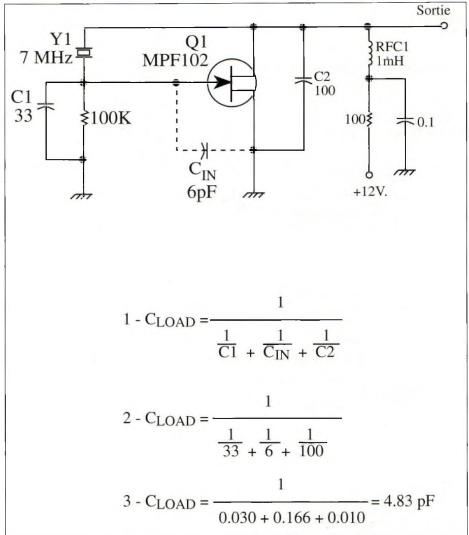
$$1 - C_{LOAD} = \frac{1}{\frac{1}{C1} + \frac{1}{C_{IN}} + \frac{1}{C2}}$$
