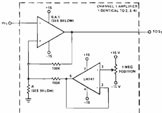
O.A. 1 IS OP AMP WITH SUITABLE BANDWIDTH, SLEW RATE, ETC. FOR DESIRED SIGNALS
