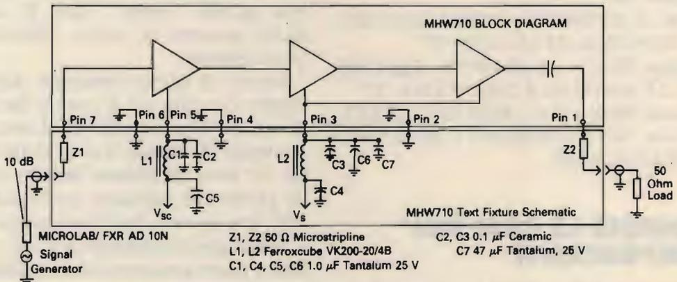
NOTE: No Internal D.C. blocking on input pin.
