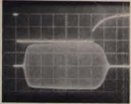
Fig. 3 — The keyed cw waveform of the Kenwood TS-180S. The horizontal divisions are each 5 ms. The upper waveform displays the actual key-down time. Such a smooth waveform should not have any clicks.
