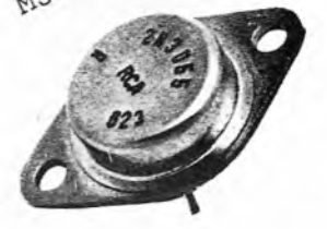
TRANSISTORS: BD709. BDX71. MJE29 ET 3055.
