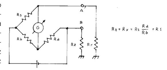
$$R_z + R_x = R_s \frac{R_a}{R_b} = R_1$$
