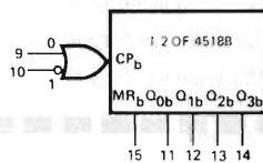
$V_{DD}$  = Pin 16
