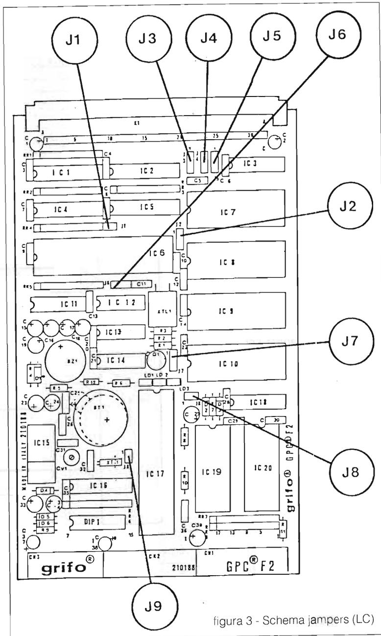
figura 3 - Schema jumpers (LC)
