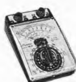
Hansen-Unitester HM 16 Innenwiderstand 20 000 \Omega /V = 5 000 \Omega /V ~ 120.-
