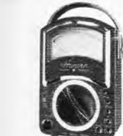
Hansen-Uni-Tester HRV 100 Eigenverbr.: 33 000 \Omega /V = 15 000 \Omega /V ~ 158.-
