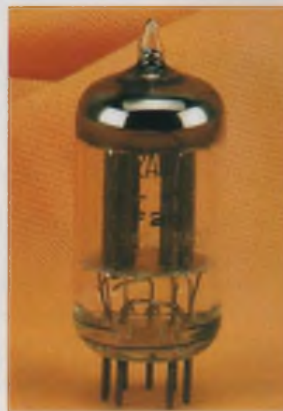
Figure 2 Embase miniature 9 broches (Noval)
