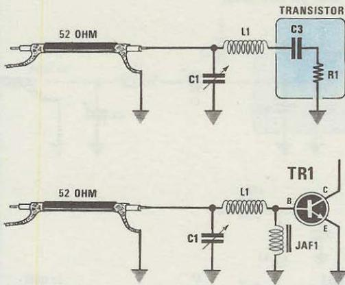
$$1^\circ XC3 = 1.000.000 : (6,28 \times \text{MHz} \times C3 \text{ in pF})$$
