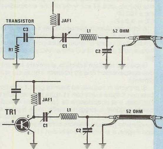
$$1^\circ XC3 = 1.000.000 : (6,28 \times \text{MHz} \times C3 \text{ in pF})$$
