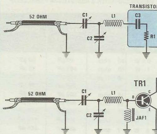
$$1^\circ XC3 = 1.000.000 : (6,28 \times \text{MHz} \times C3 \text{ in pF})$$
