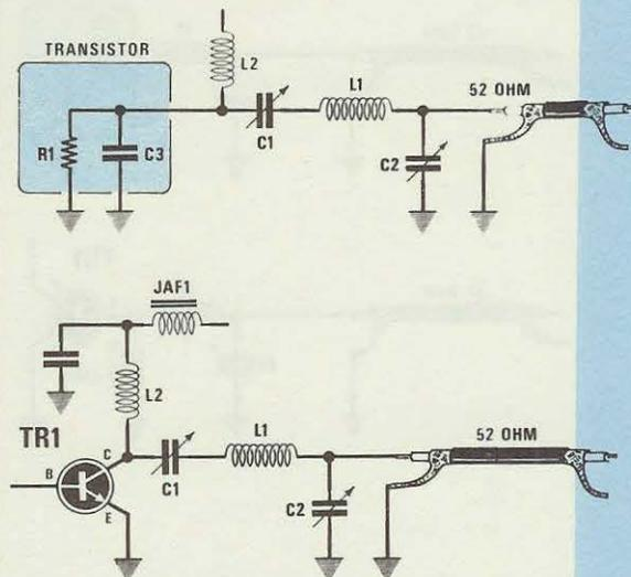
1°  $XC3 = 1.000.000 : (6,28 \times \text{MHz} \times C3 \text{ in pF})$
