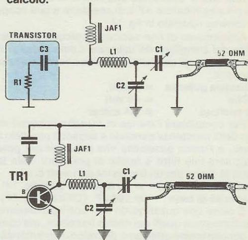
$$1^\circ XC3 = 1.000.000 : (6,28 \times \text{MHz} \times C3 \text{ in pF})$$
