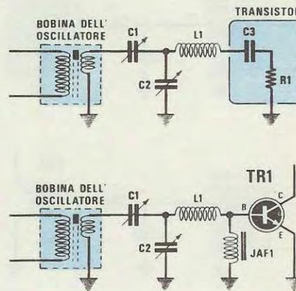
$$1^\circ XC3 = 1.000.000 : (6,28 \times \text{MHz} \times C3 \text{ in pF})$$
