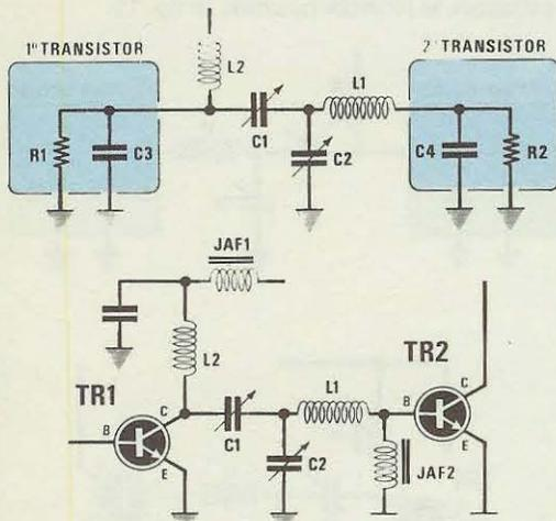
1°  $XC3 = 1.000.000 : (6,28 \times \text{MHz} \times C3 \text{ in pF})$
