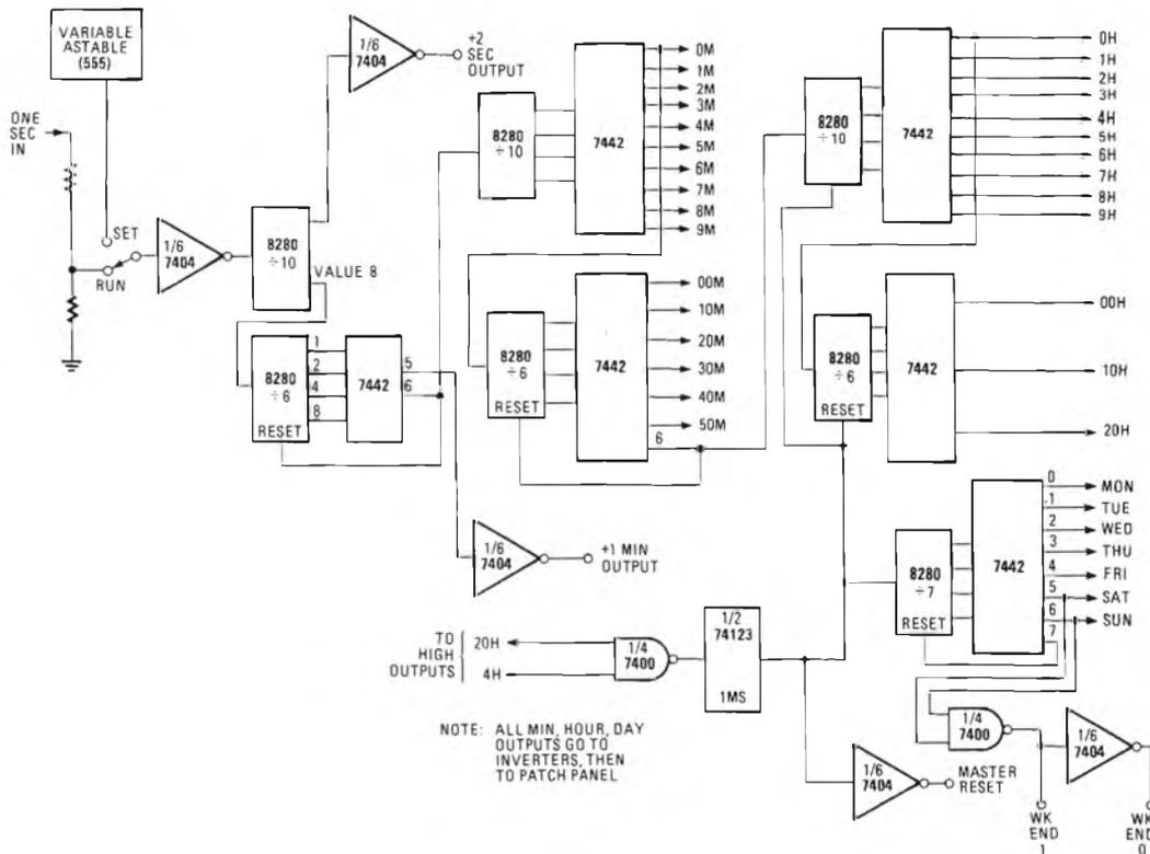
NOTE: ALL MIN, HOUR, DAY OUTPUTS GO TO INVERTERS, THEN TO PATCH PANEL
